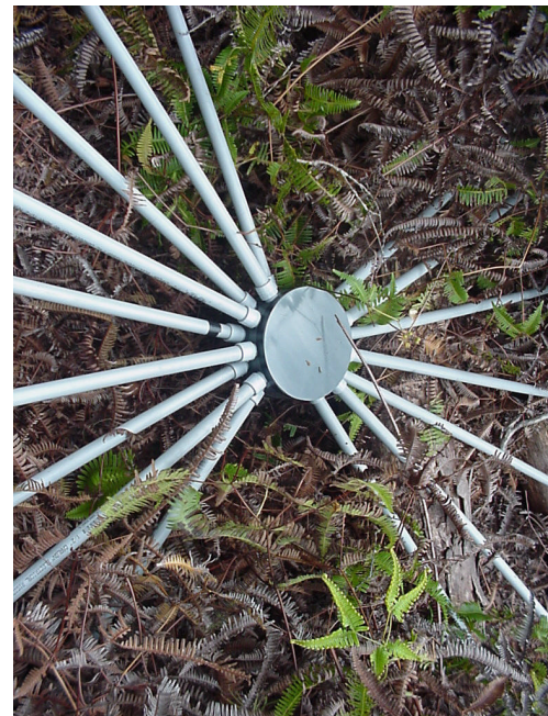
Figure 9. Wind-noise-reducing pipe array design (left) and PVC implementation (right).
