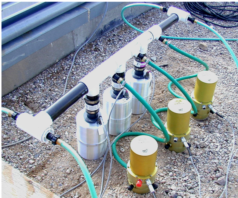
Figure 4 – MB2000 and Chaparral 5 Comparison Test at Sandia FACT Site
