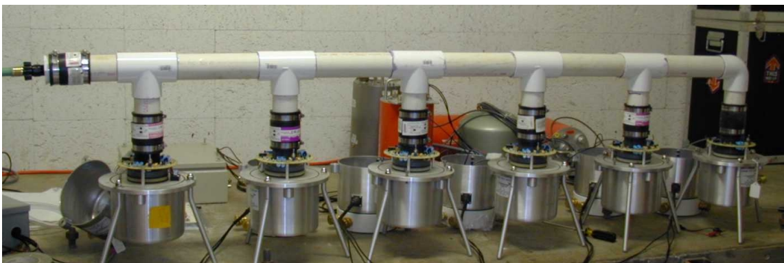
Figure 2 – Reference Sensor (left) and Five IS-59 Acoustically Paralleled Chaparral 5 Production Sensors
