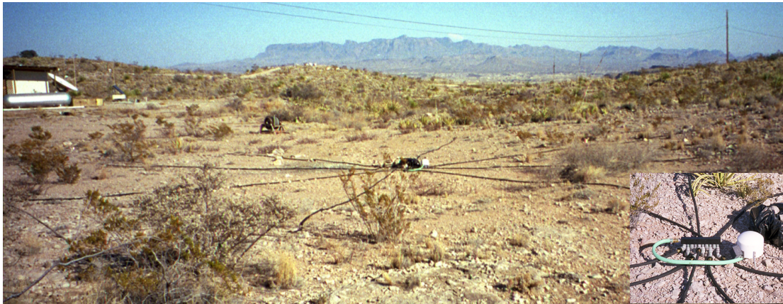
Figure 5: One element of a regional infrasound array. The porous hoses are summed by the manifold shown in the lower right, which is connected to the Chapparel Model 2 microphone.
