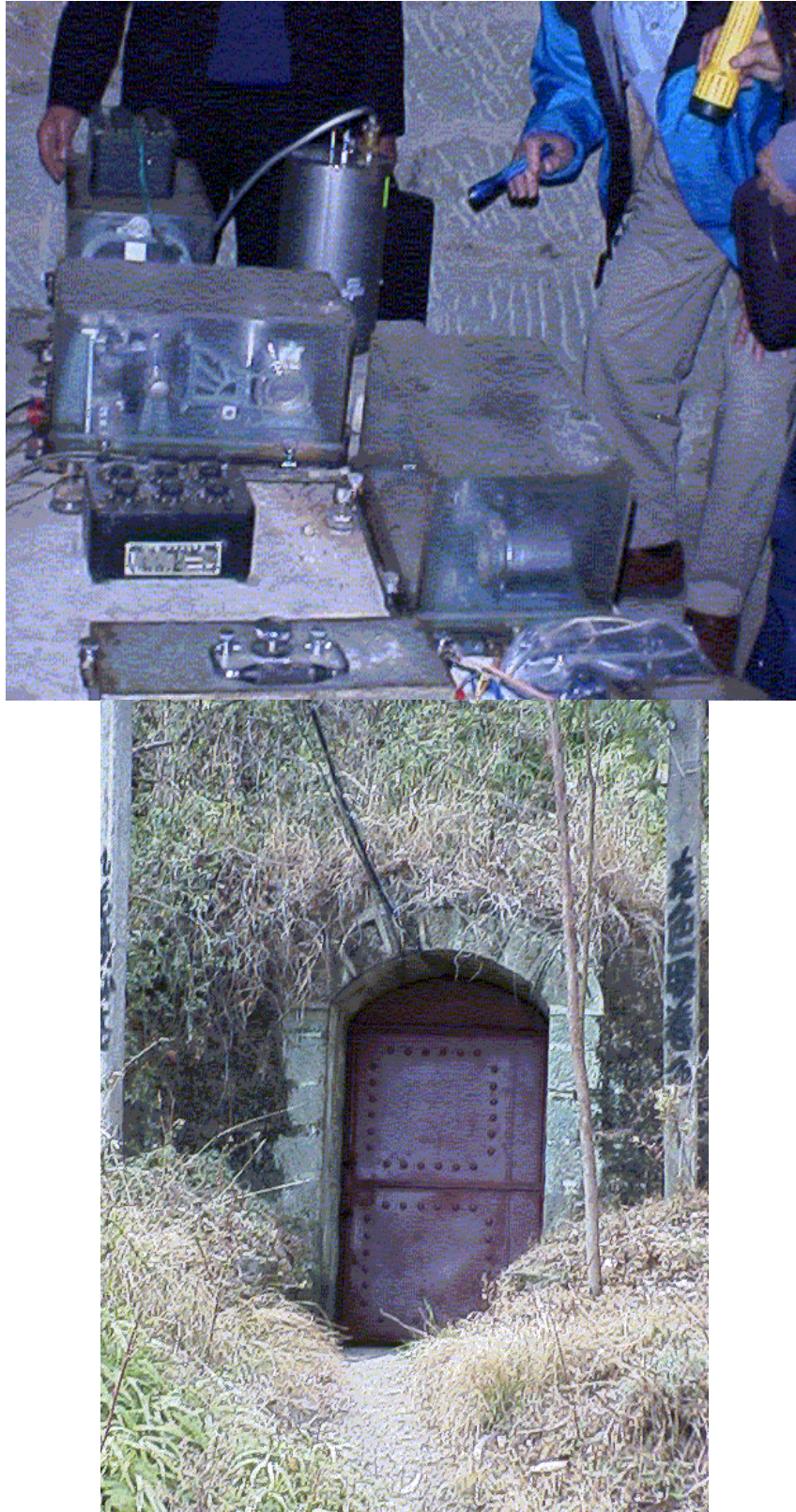
Figure 3(a): Top – Broad-band instruments installed side by side to short-period Chinese SK-type instruments Figure 3(b): Bottom – Entrance to vault housing the seismic instruments at one site in Yunnan, China
