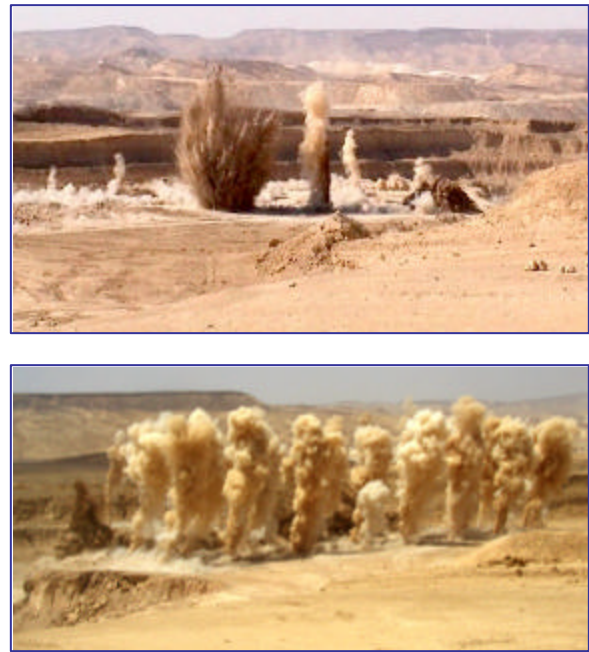
Figure 9. Experimental blasts by the “onion” method at Rotem quarry (Negev). Upper photo shows initial small shots, to create near-spherical cavities (“onions”), used for the 25-ton calibration shot on 12/5/2002 (down photo).
