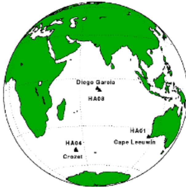
Figure 1. IMS Hydroacoustic Station Locations. Each triangle represents a triad of hydrophones. The current operational instruments are the two triads at Diego Garcia and the single triad at Cape Leeuwin. The two triads at Crozet are scheduled to come online in spring, 2003.
