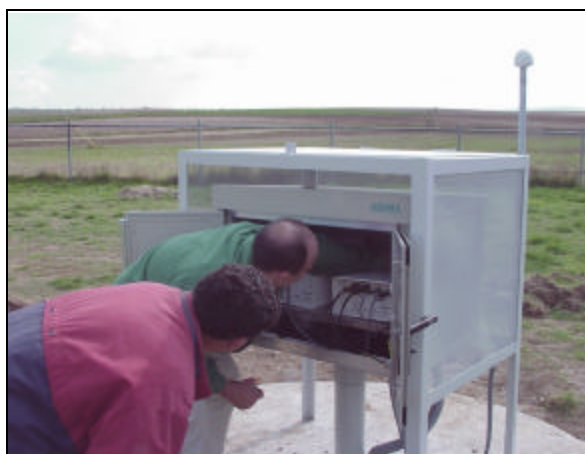
Figure 5. New WTU with shade cover, external GPS antenna shown in upper right of picture.
