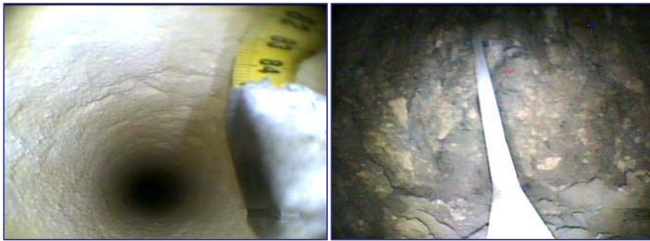
**Figure 12.** Snapshots of the GeoVISION borehole camera video-records show a borehole inner view before (left) and after (right) a small preparatory explosion. The measuring strip (~80 cm length) attached to the camera is exposed as almost straightened over the created cavity bottom.
