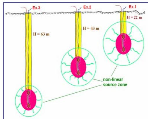
**Figure 13.** Schematic view of supposed diverse non-linear zones for explosions at different depths.
