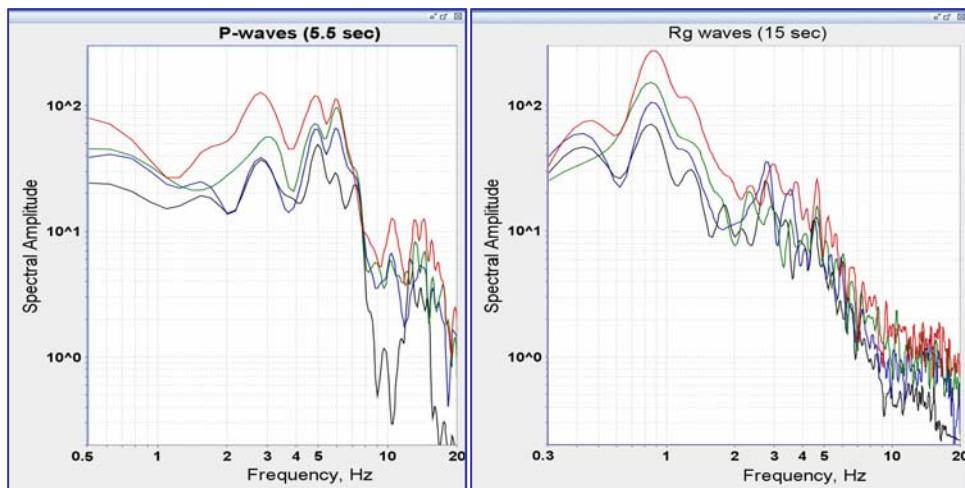
**Figure 6.** Spectra of P waves and surface waves (Rg) at EIL (vertical) for 4 explosions (the data were pre-filtered in the 0.5-20 Hz band). Curve colors fit the seismograms on Figure 5.
