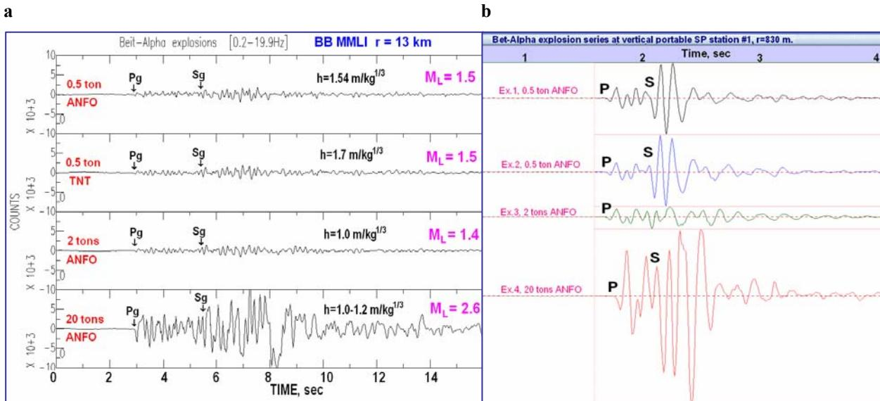
**Figure 10. Seismograms (in absolute scale) of Bet-Alpha shots show reduced amplitudes and magnitudes under insufficient scaled charge depth  $h$  at close BB (a) and portable SP station at ~1 km (b).**
