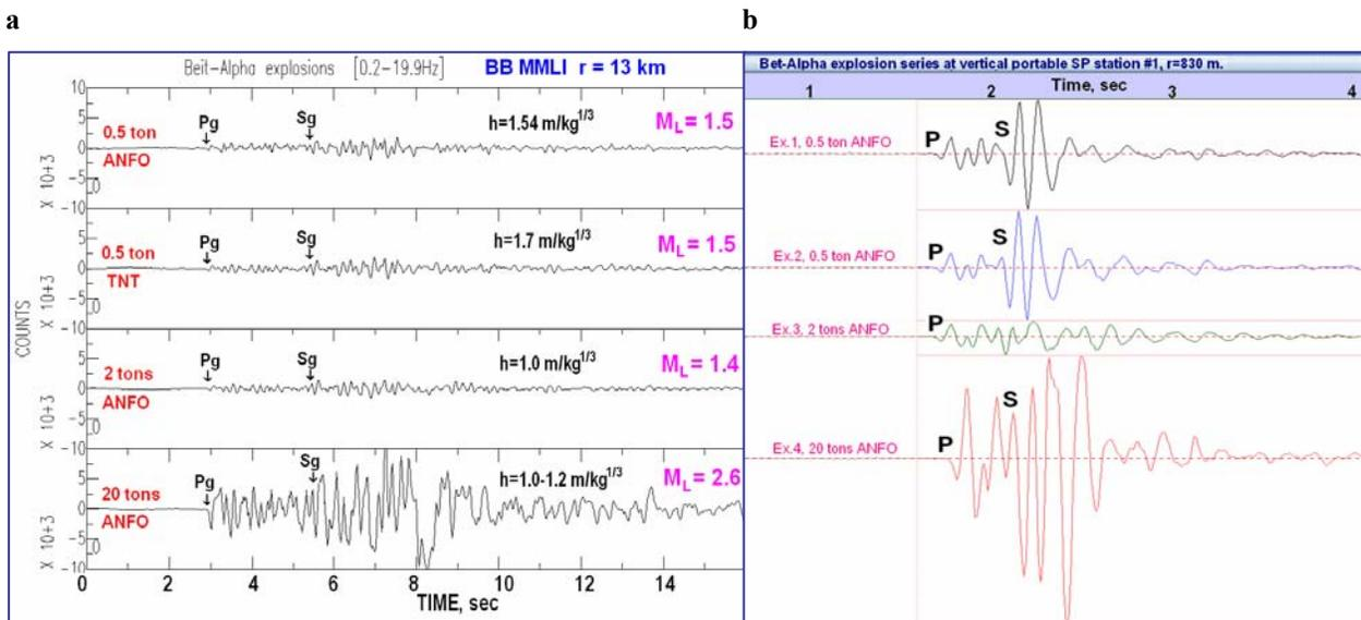
**Figure 10. Seismograms (in absolute scale) of Bet-Alpha shots show reduced amplitudes and magnitudes under insufficient scaled charge depth  $h$  at close BB (a) and portable SP station at  $\sim 1$  km (b).**
