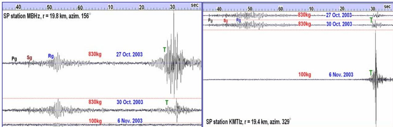
Figure 4. Observations of diverse acoustic phases (T) from surface shots in 2003 at two ISN seismic stations (plotted in absolute scale, filter 1-15 Hz is applied).
