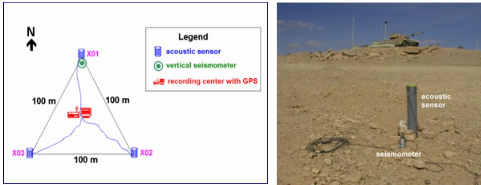
**Figure 3. Observations in 1998: (a) Configuration of a hybrid seismic/acoustic portable tripartite array; (b) installed sensors in the Northern apex of the station triangle during one of the shots.**
