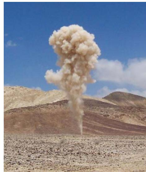
**Figure 14.** A trial shot (~300 kg ANFO) in a hole with depth 63 m. Ejection of gases and dust lasted ~30 sec, a cavity of ~3m size was created.
