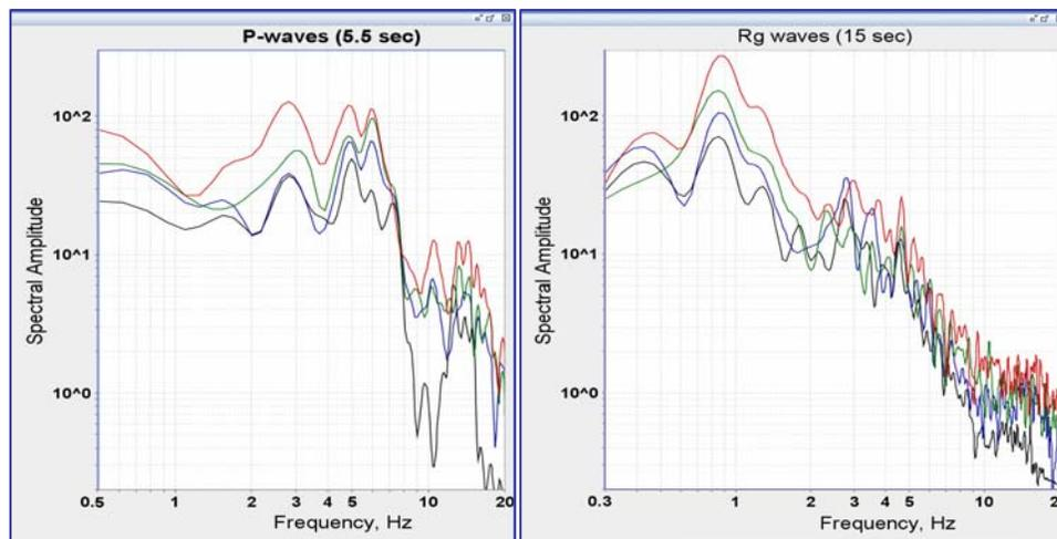
Figure 6. Spectra of P waves and surface waves (Rg) at EIL (vertical) for 4 explosions (the data were pre-filtered in the 0.5-20 Hz band). Curve colors fit the seismograms on Figure 5.
