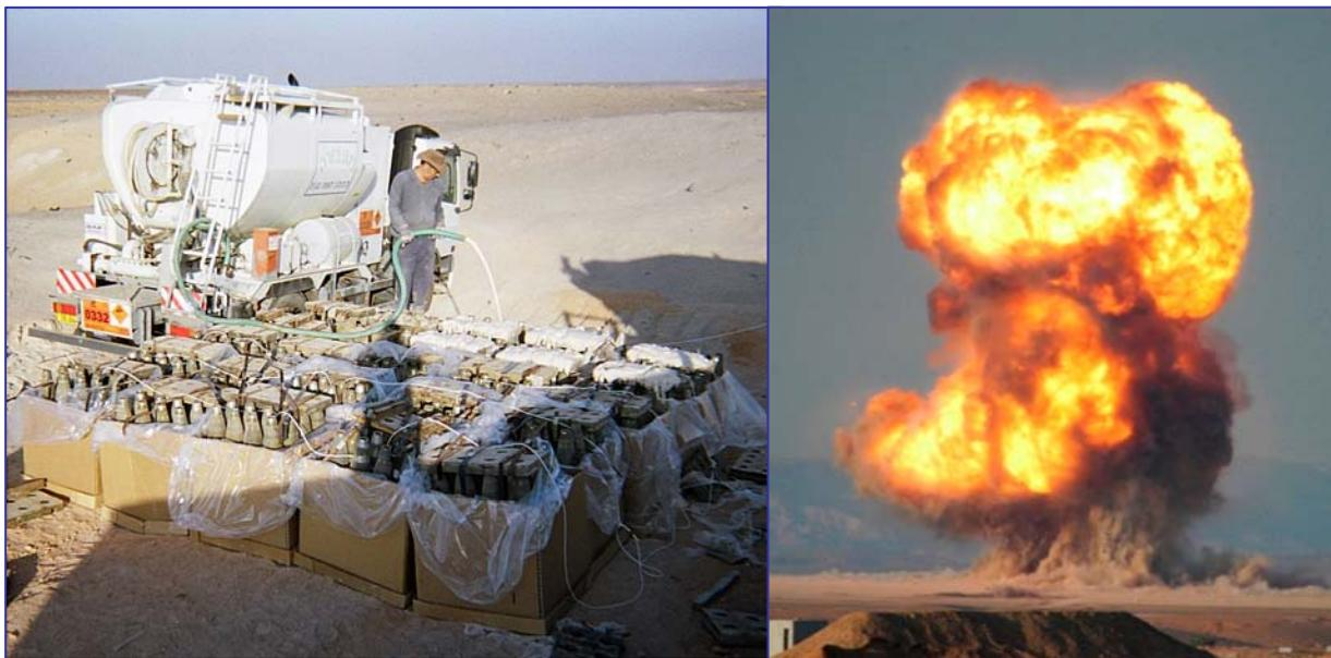
**Figure 2. Sayarim ammunition explosion on Dec. 6, 2005 (Ex.17). Industrial explosive (ANFO-like emulsion Henamit) was added to provide full demolition of the shells (left). The right photo is made from a distance ~3 km, with a large zoom (courtesy of Y. Hamashdyan of IDF).**
