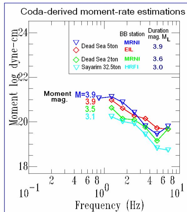
**Figure 11. Coda-magnitude estimations for large-scale calibration explosions conducted by GII.**
