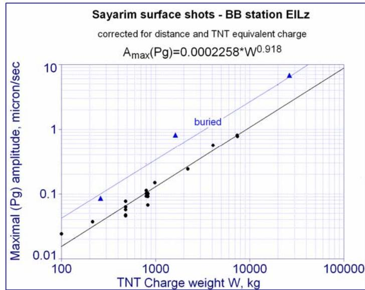
Figure 7. Yield scaling of surface seismic sources at BB station EIL. Data of 3 buried (borehole) Sayarim experimental explosions (2004) at EIL are also shown for comparison (▲).
