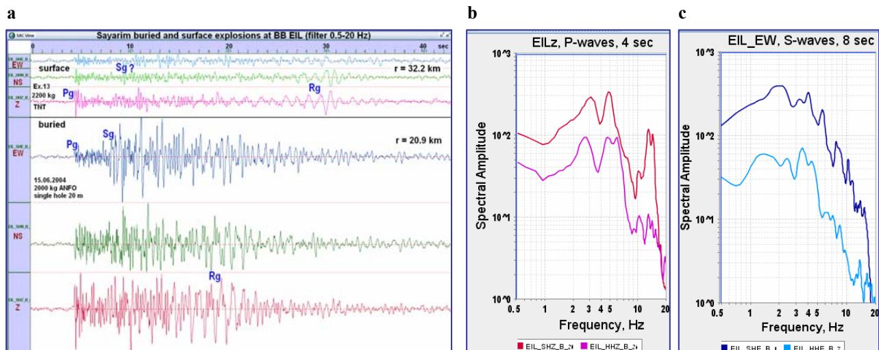
**Figure 8.** Seismograms in absolute scale (a) and spectra of Pg (b) and Sg (c) for surface and buried shots at EIL. Spectra colors fit appropriate seismograms.
