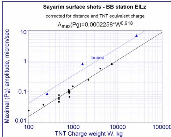
**Figure 7.** Yield scaling of surface seismic sources at BB station EIL. Data of 3 buried (borehole) Sayarim experimental explosions (2004) at EIL are also shown for comparison ( $\blacktriangle$ ).
