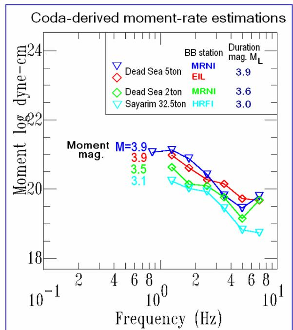
**Figure 11. Coda-magnitude estimations for large-scale calibration explosions conducted by GII.**
