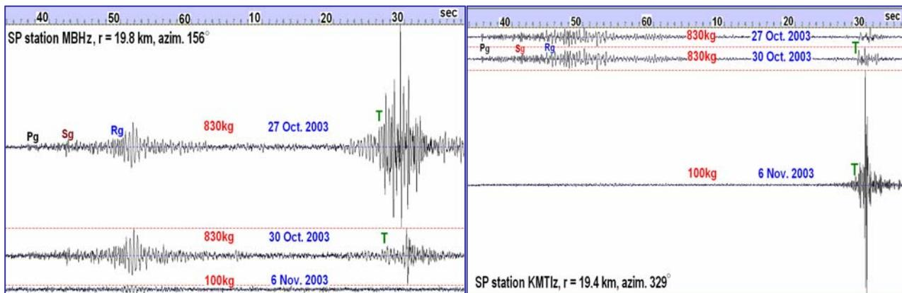
**Figure 4. Observations of diverse acoustic phases (T) from surface shots in 2003 at two ISN seismic stations (plotted in absolute scale, filter 1-15 Hz is applied).**
