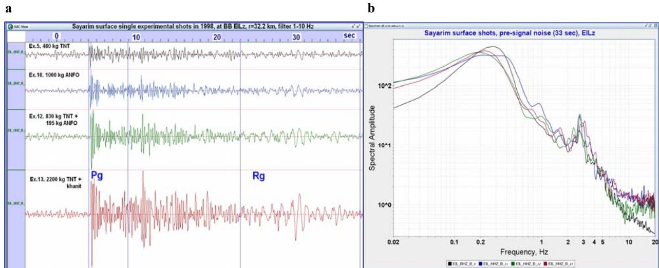
**Figure 5. (a)** Seismograms (in absolute scale) of 4 selected Sayarim surface explosions at BB station EIL (vertical), low-frequency noise ( $f < 1$  Hz) is filtered, vertical lines show windows for spectral analysis; **(b)** spectra of pre-signal noise (curve colors fit the appropriate seismograms).
