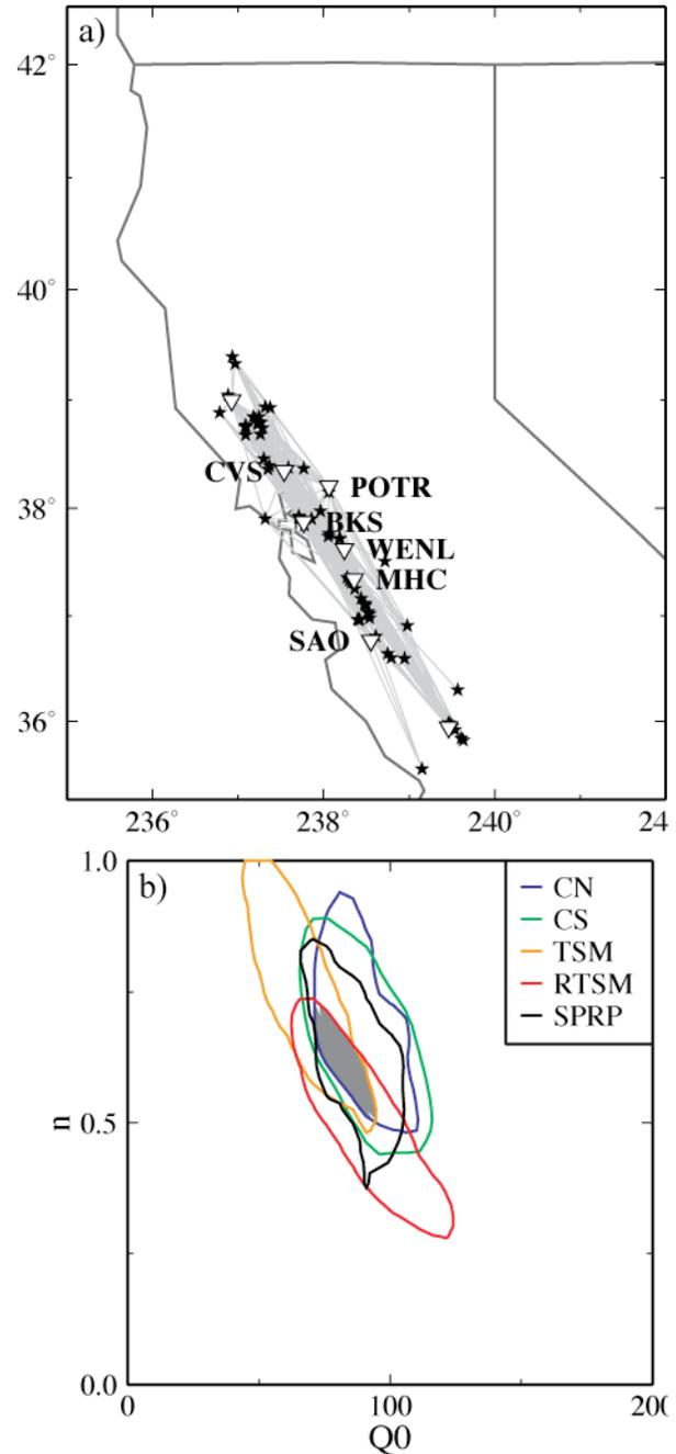
**Figure 2. Method comparison. (a) Map (same region as Figure 1) of the subset used in the comparison analysis. Data are in a small region near the San Francisco Bay Area, primarily along the Franciscan block. (b) Power-law parameters and their empirical 95% confidence regions are given. The intersecting region is shaded grey.**
