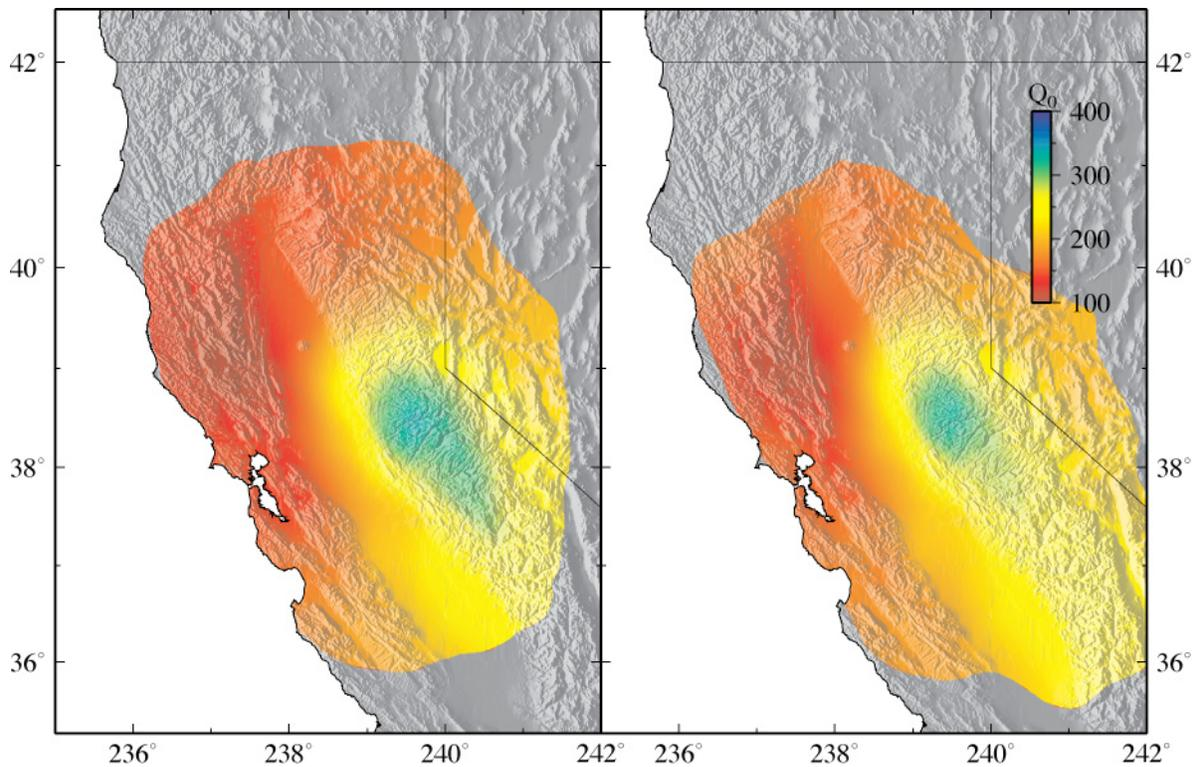
**Figure 5. Attenuation tomography using amplitudes (a) where the source and site term is solved for in the inversion and (b) where the source term is removed from the amplitudes using a coda-derived moment rate.**
