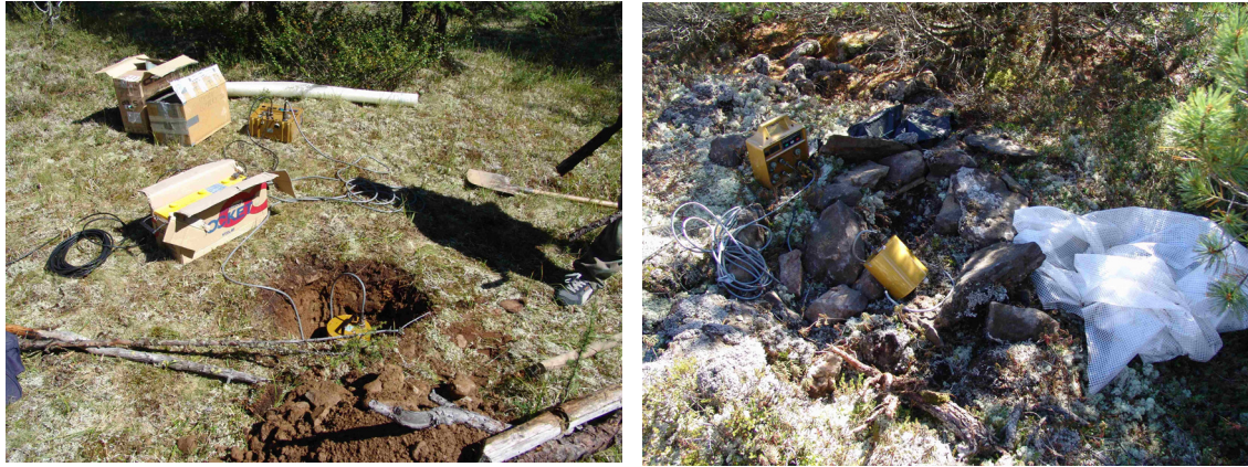
Figure 3. Left - Typical station installation consisting of a Geotech Instruments KS-2000 broadband seismometer, Smart24 digitizer, and large battery. Right – A seismic station shown as found after destruction by a bear. The bear removed all station coverings and batteries and extracted the seismometer from its posthole.
