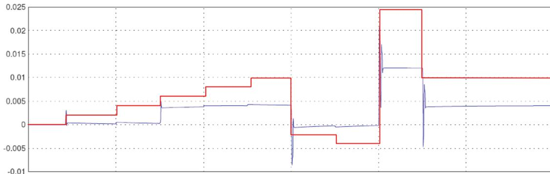
**Figure 9. Simulation of combined closed and open loop operation of the  $\mu$ Seis in response to a stepped input over a 30s period. The input is in red, the position of the proof mass is in blue, showing operation at displacements of 0, 1 and 3 multiples of the LCAT period.**
