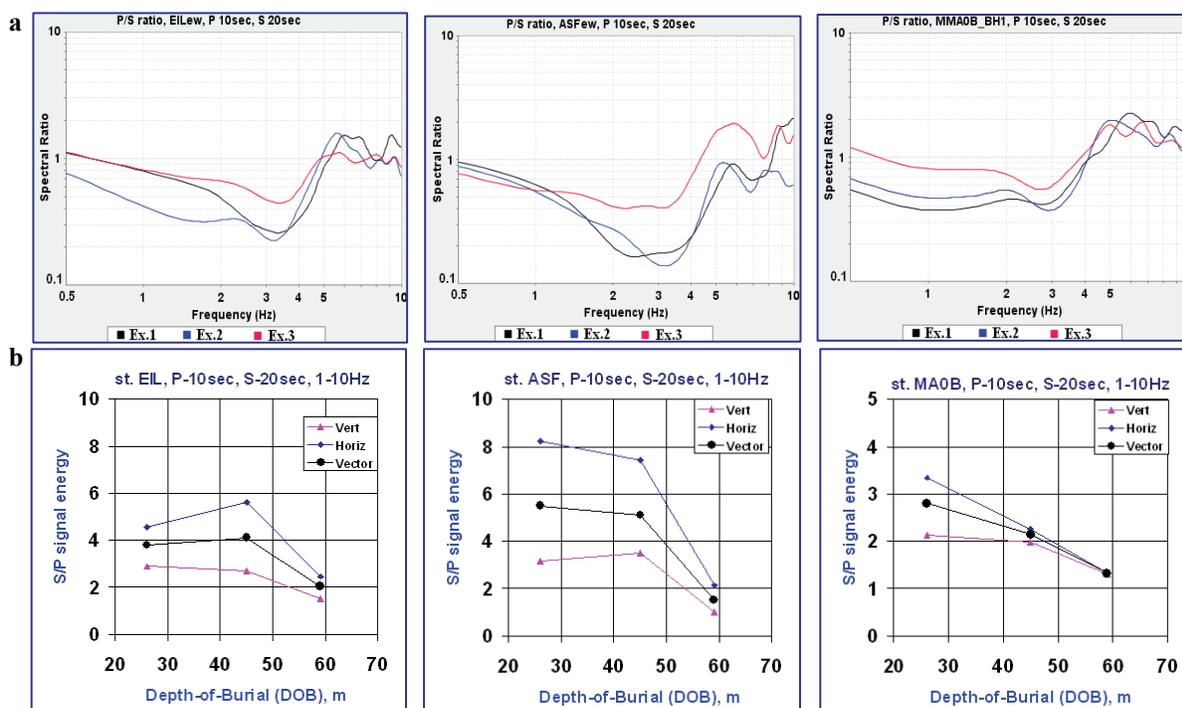
Figure 15. Energy partition at near-regional distances: spectral ratios P/S show decreased S-wave excitation for deeper shots in the range ~0.5–8 Hz (a); signal energy ratios S/P decrease, in general, monotonous with depth (b).
