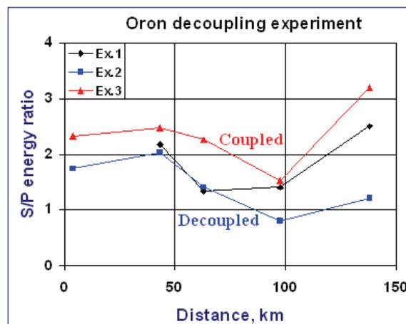
Figure 6. Energy partition estimation: S/P energy ratio for the Decoupling series shots.
