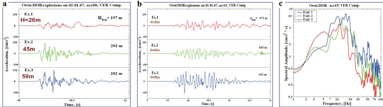
Figure 8. Vertical accelerograms at close station ACC00 equidistant from 3 DOB shots (a), and the remotest station ACC15 (b) and amplitude spectra (c). Hypocentral distances to the shots are shown.
