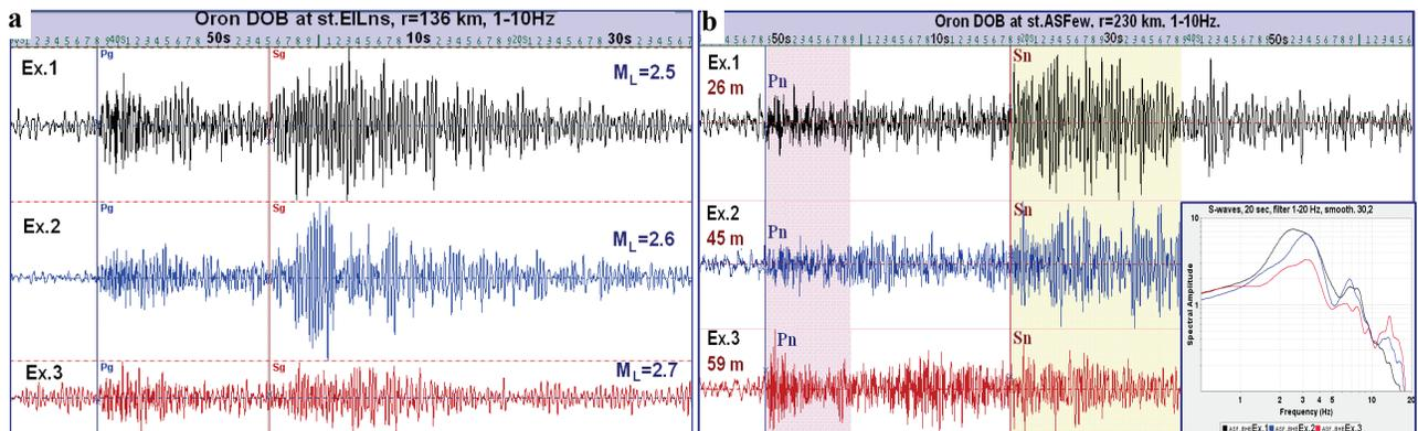
Figure 11. Horizontal seismograms (in absolute scale) at two IMS BB stations: EIL-NS (Radial) component (a), ASF-EW (~Transversal) component, windows for calculation spectra and spectral ratio are shown; conversion of spectra dominance for different shots at  $\sim 10$  Hz is observed (b).
