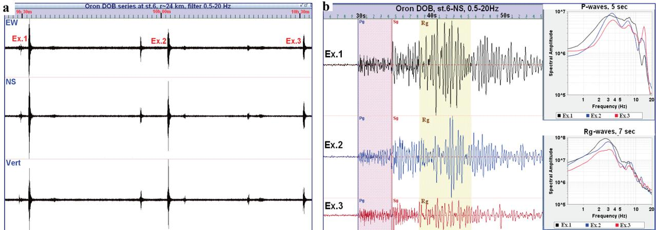
Figure 10. Close local recordings (in absolute scale) at the central 3C station of the SP tripartite array (St.6) at  $r \sim 24$  km: continuous 3C recording section of all 3 shots (a), NS records and spectra of P and Rg phases (b). A clear Rg onset is observed at vertical records (velocity  $\sim 2$  km/s). Note a dominant spectral peak for Ex.3 at 13-15 Hz in P-phase which is not observed in Rg-phase.
