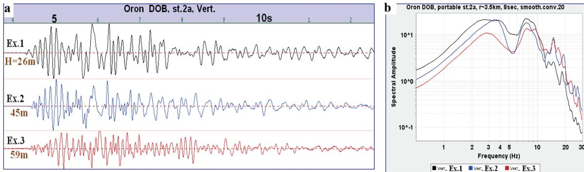
Figure 9. Vertical seismograms in absolute scale (a) and spectra of the whole signal (8 sec) (b) at the closest SP station at  $r \sim 3.5$  km. Note dominant energy for the deepest Ex.3 at high frequencies  $f > 10$  Hz.
