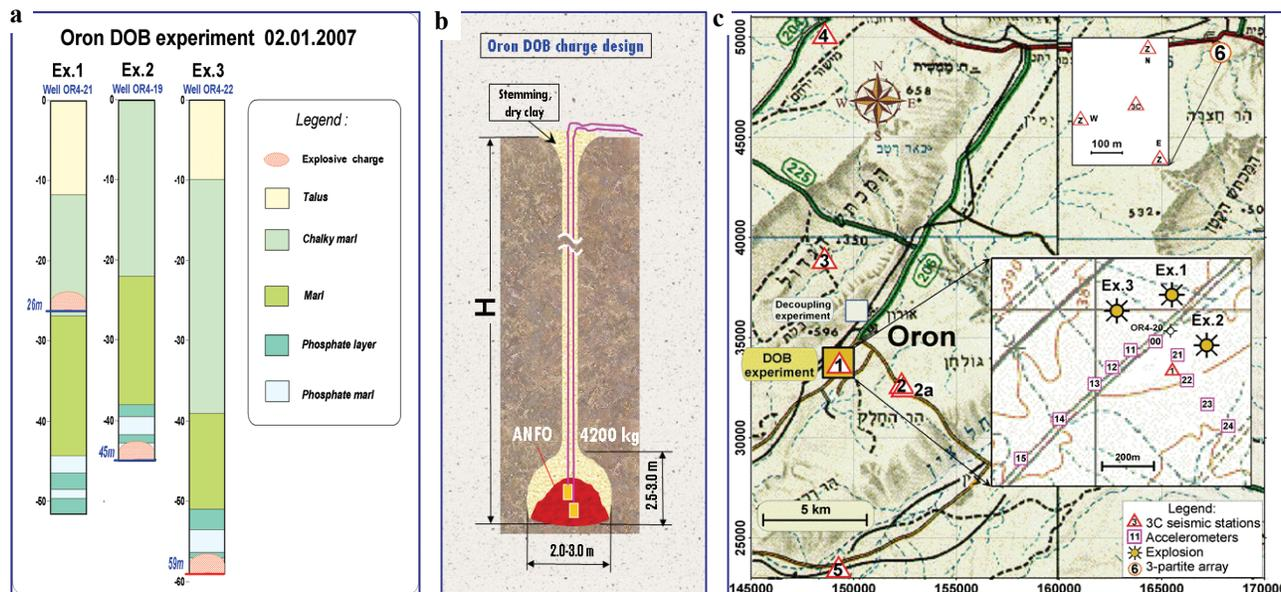
Figure 7. Geology of explosion boreholes from drilling logs (a); specific charge design providing large near-spherical seismic sources (b); location of the two experiment sites and portable stations, two insertions show detailed location of the tripartite array elements (st.6) and configuration of the explosion boreholes and accelerometers (c).
