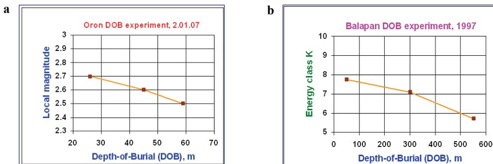
Figure 12. Magnitude versus source depth for two DOB experiments: local (duration) magnitude  $M_L$  at Oron (a) and Energy class K at Balapan (b).
