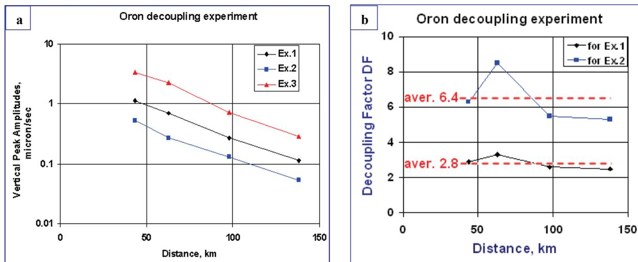
Figure 5. Signal peak amplitude (a) and Decoupling Factor (b) in a broad distance range for the partially decoupled explosions in soft sediment media.
