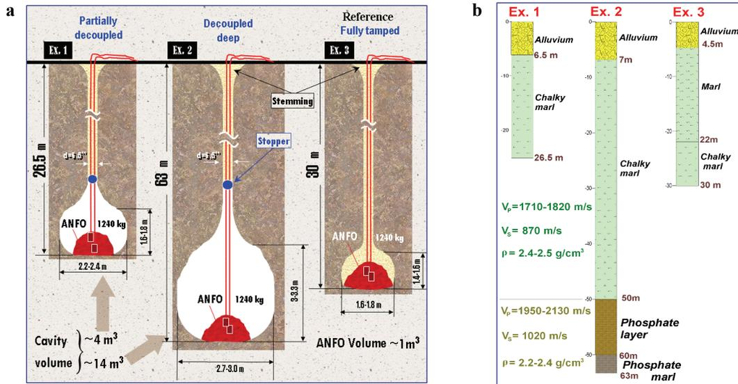
Figure 2. Design of the Decoupling experiment (a) and the site geology from the shot borehole drilling logs (b).
