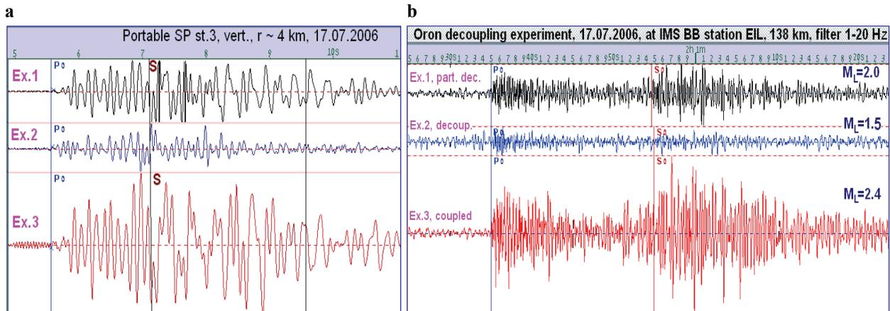
Figure 4. Vertical seismograms in absolute scale at close (a) and near-regional (b) distances.
