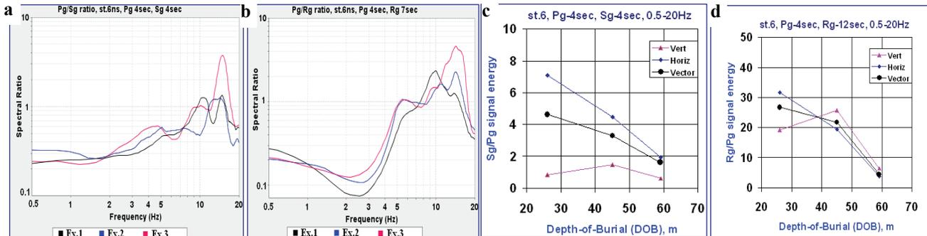
Figure 14. Energy partition at close local station st.6 (24 km): spectral ratios Pg/Sg (a) and Pg/Rg (b) suppose a weak dependence on source depth at 2–5 Hz; signal energy ratios Sg/Pg (c) and Rg/Pg (d) show an obvious decrease for deeper shots, especially for the Horizontal (EW+NS) component.
