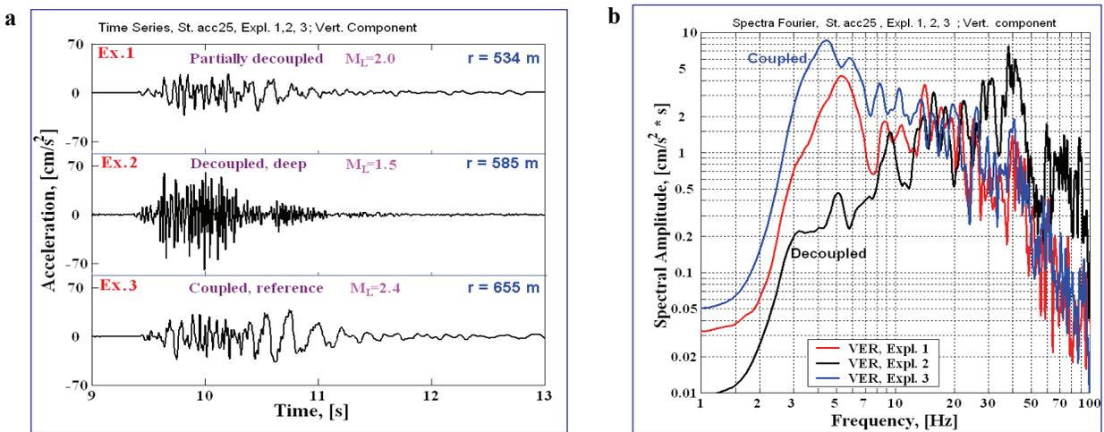
Figure 3. Vertical signal records (a) and spectra (b) at ~0.6 km (accelerometer ETNA). Local (duration) magnitudes  $M_L$  and epicentral distances are also shown.
