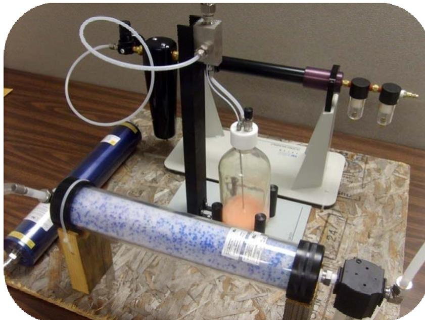
**Figure 3. Assembled aerosol generation apparatus.**
