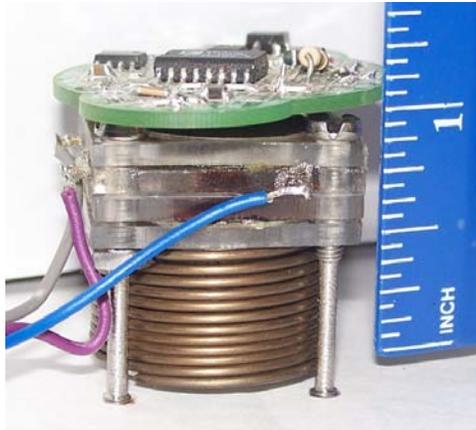
**Figure 6. Prototype sensor with electronics.**
