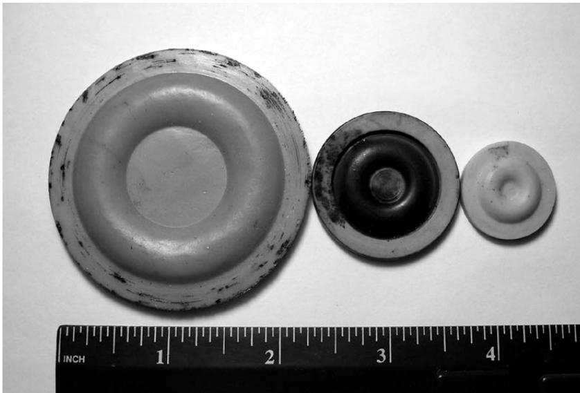
**Figure 3. Standard membrane and two designs of a shrunken membrane.**
