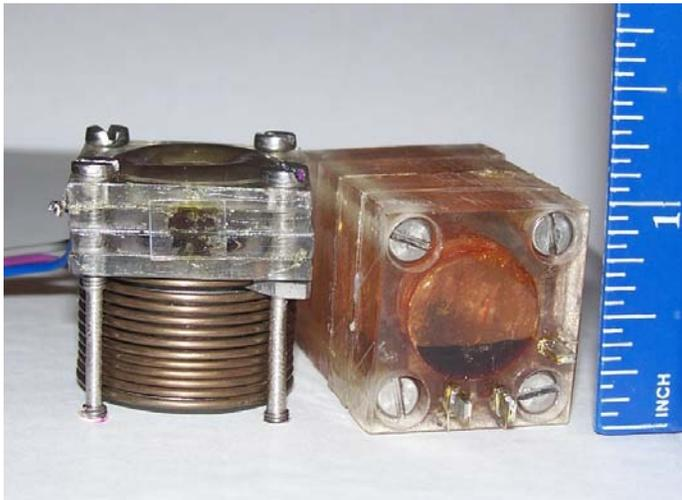
**Figure 5. Vertical and horizontal/rotational prototype sensor assemblies.**
