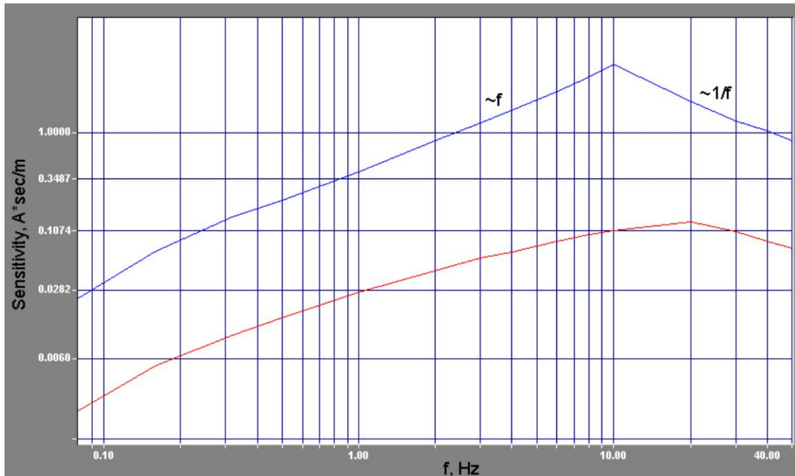
**Figure 4. Effect of the additional inertial mass (blue) on a Proto 1 (red) sensitivity and form of the frequency response.**
