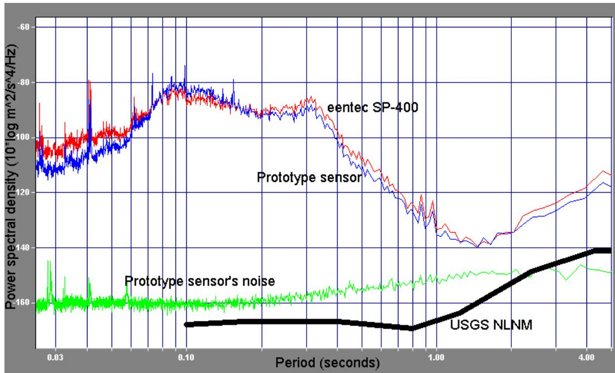
Figure 7. Signal and noise spectra of a prototype sensor.
