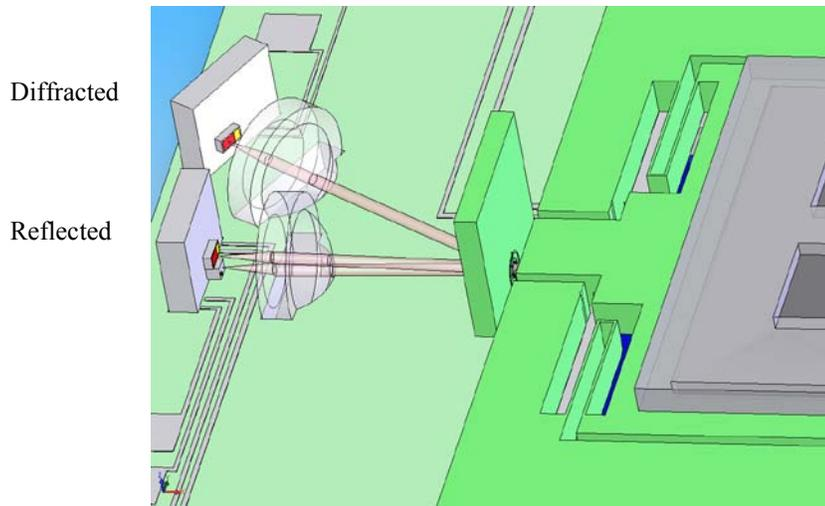
Figure 4. Laser and two photo diodes.
