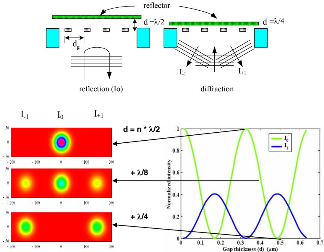
**Figure 3. Images in the lower section show the variations in intensity of reflected and diffracted orders with the gap between the grating and reflector.**
