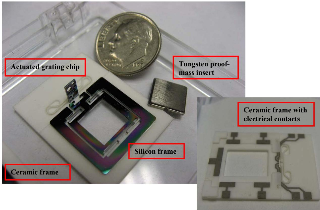
Figure 5. MEMS seismometer components.
