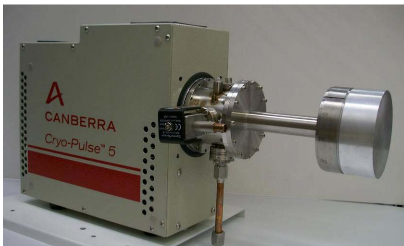
Figure 4. Mock-up of the complete UHV Cryo-Pulse® 5 with test end cap.
