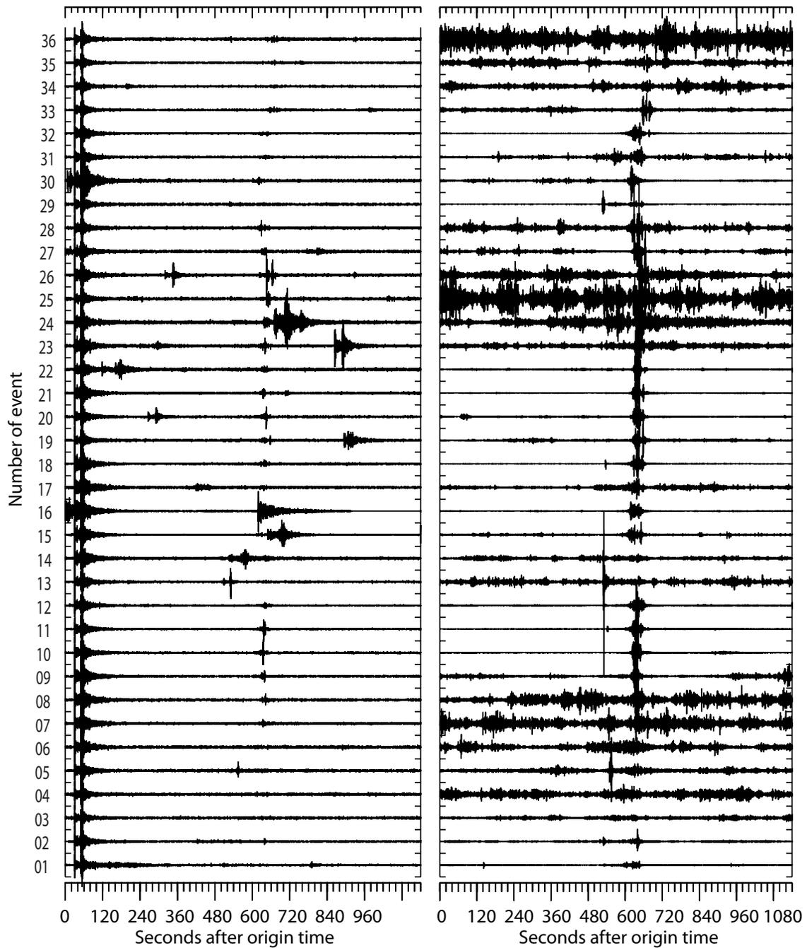
Figure 2. Waveforms from the short-period vertical seismic sensor ARA1\_sz (left) and the co-located microbarograph sensor ARA1\_BDF (right) for the Finnish explosions during 2008. The same vertical scale is applied to all of the traces within each panel. All waveforms are bandpass filtered between 2 and 7 Hz.
