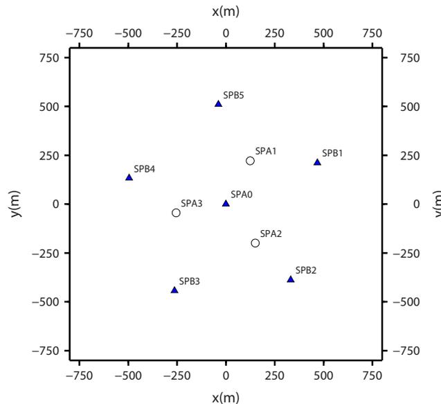
Figure 7. Map showing the configuration of the Spitsbergen array (SPITS). The blue triangles are three-component stations.
