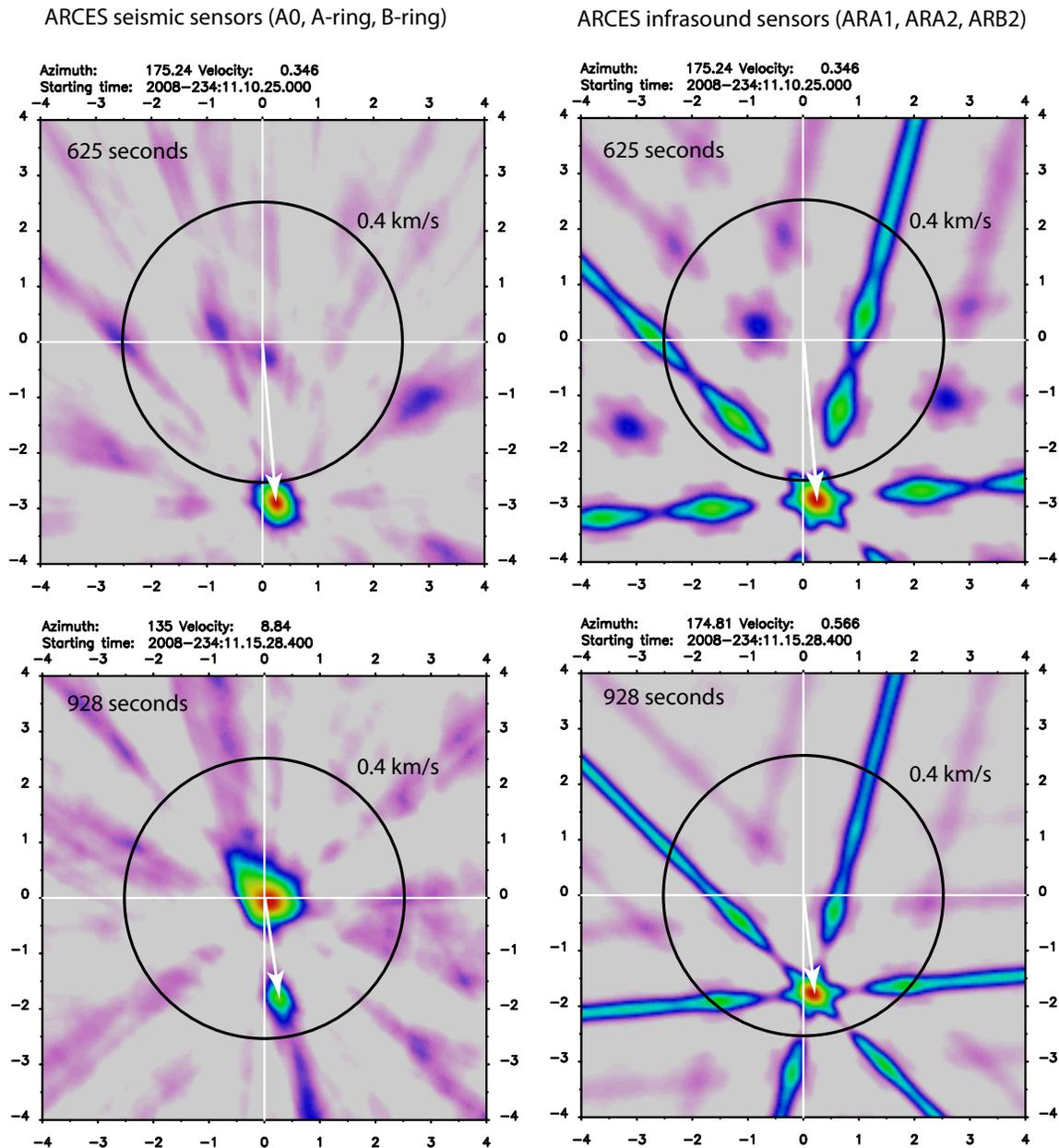
**Figure 3. Slowness estimates at 625 seconds (above) and 928 seconds (below) after the explosion at 11:00 UTC on August 21, 2008. For the seismic estimates (the two plots to the left), only the innermost nine sites of the ARCES array are used. The seismic estimate for the later arrival (lower left panel) indicates an apparent velocity consistent with seismic wave speed, although evidence is seen for energy arriving with sound speed. The circles correspond to an apparent velocity of 0.4 km/s.**
