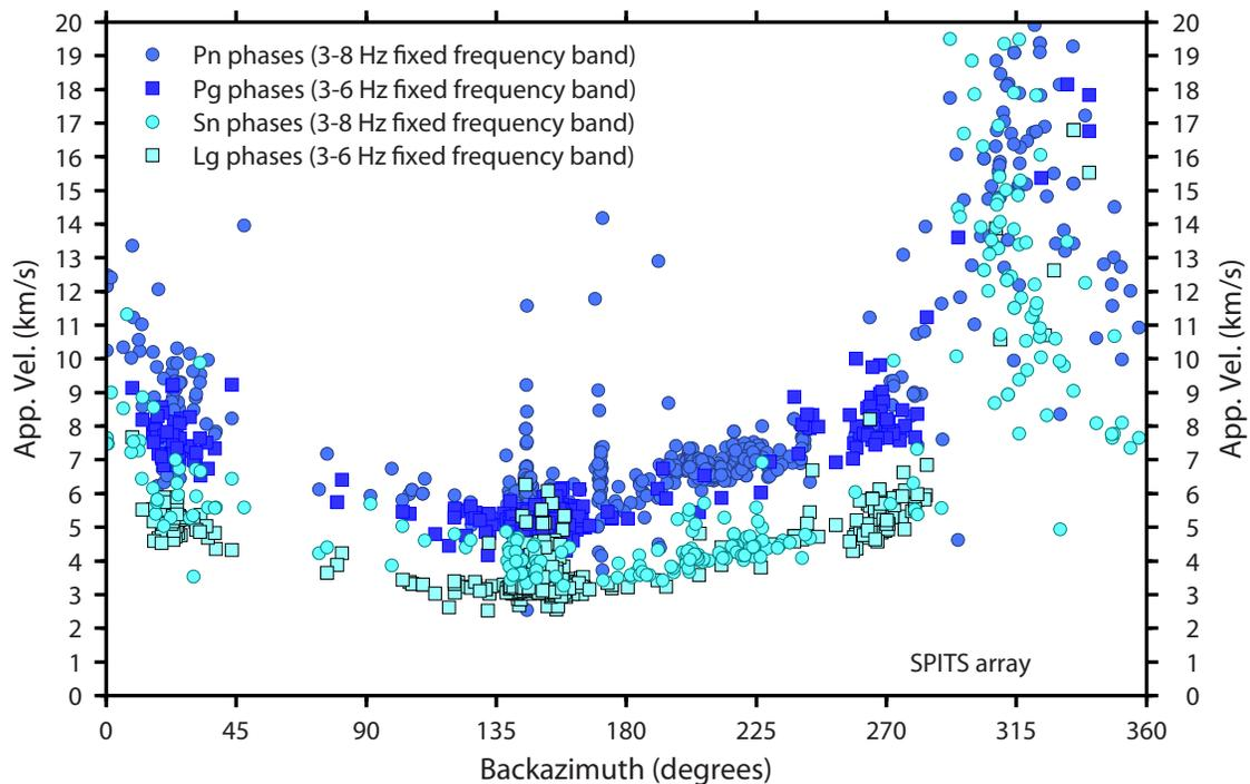
**Figure 8. Apparent velocity of regional phases recorded by the SPITS array as a function of geographical backazimuth. The backazimuths are based on the solutions in the NORSAR analyst-reviewed regional bulletin. The slowness estimates have been made by fixed band f-k analysis as indicated, using only the vertical seismometers. The plot does not take into account epicentral distance and does not show SPITS backazimuth deviations relative to the reference backazimuth.**
