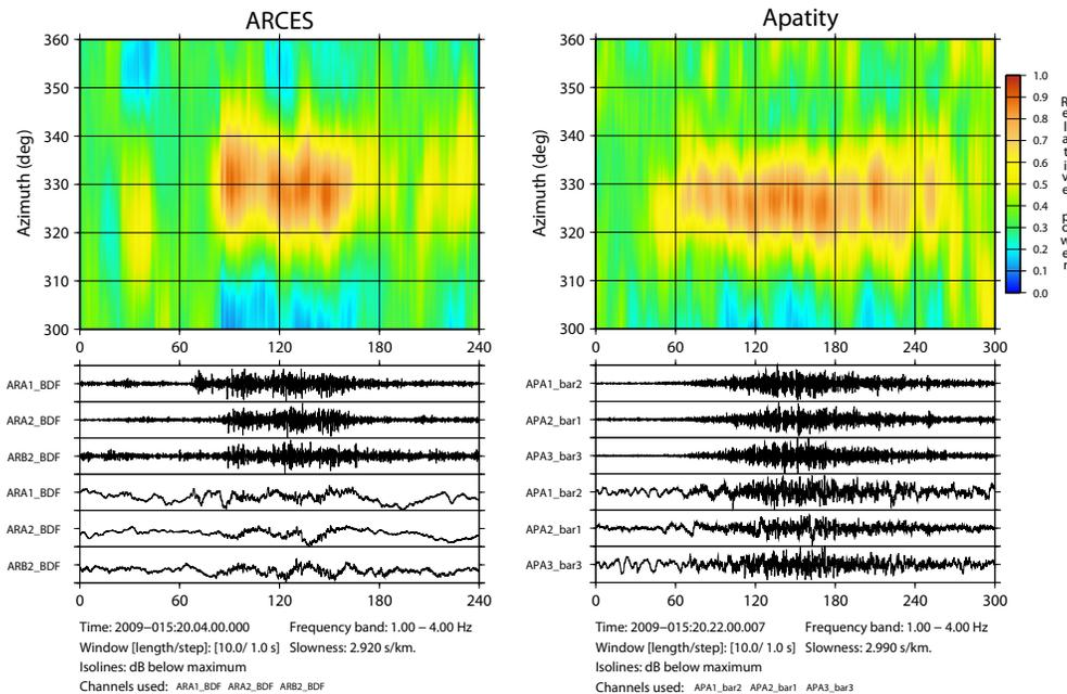
**Figure 4. Azimuthal vespagrams from analysis of ARCYES and Apatity infrasound data for the time interval around the signals from the meteor on 15 January 2009. The upper three traces of each panel show the bandpass filtered waveforms, whereas the three lower traces show the raw data. Notice that different time scales are used for the two stations. A constant slowness close to 3 s/km has been used when calculating the azimuthal vespagrams.**
