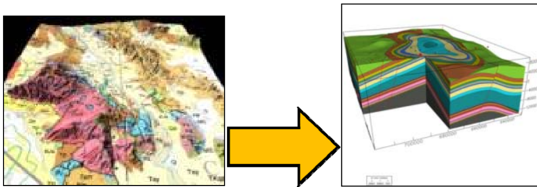
Figure 2. A variety of geologic and geophysical data will be combined to create a geologic framework model for the Source Physics Experiments in Climax Stock granite.
