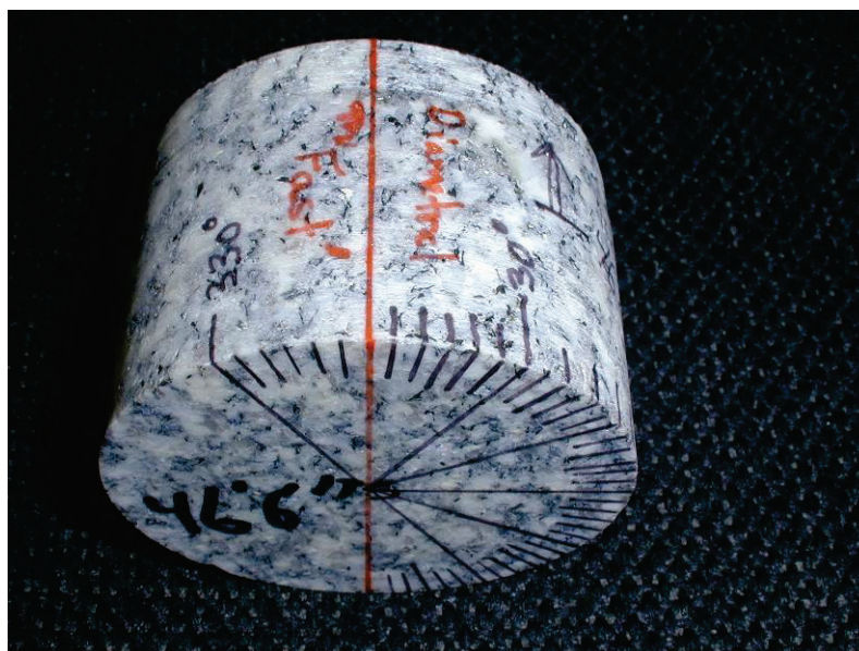
Figure 3. Barre granite core that has been partitioned every 5 degrees in order to determine the fast and slow directions of the anisotropy or “rift.”
