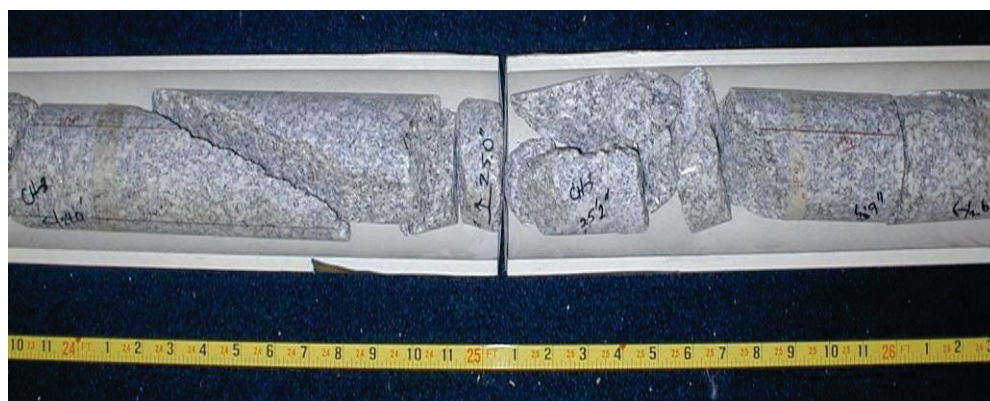
Figure 8. Examples of meso-scale damage observed in cores above the working explosion point.
