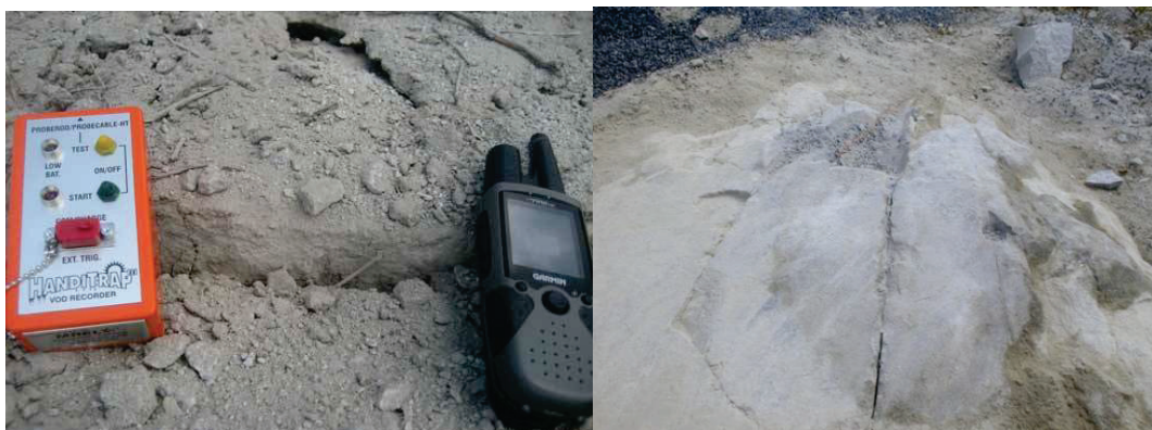
Figure 1. Radial crack formation from the Black Powder Shot 1 (left) and the Heavy ANFO Shot 2 (right).
