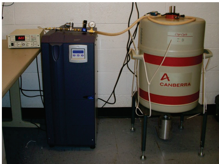
Figure 5. LN Level Controller, N_2 generator, and Cryo-Cycle ™ test setup.
