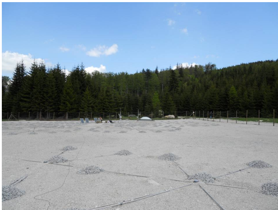
Figure 3. View from near the center of the hexagonal elements toward the rosette elements. The pad on which the four I99 elements are installed is clear of all vegetation. The forested area starts somewhat outside the fenced pad.
