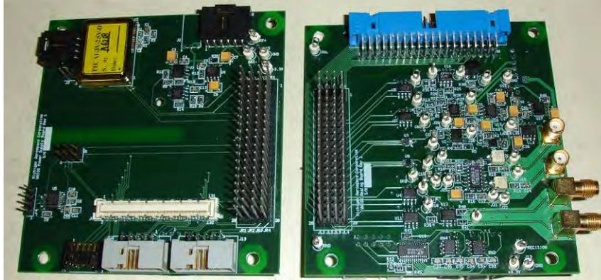
**Figure 6. Photograph of the electronics boards, power supply board (left) and analog interface board (right).**
