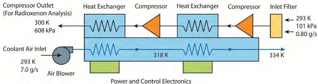
**Figure 2. Compressor system schematic.**
