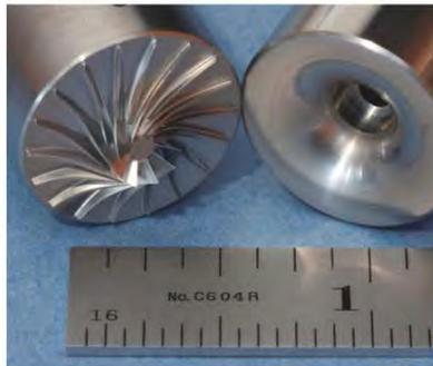
Aerodynamic Features for 400 W Compressor Impeller
