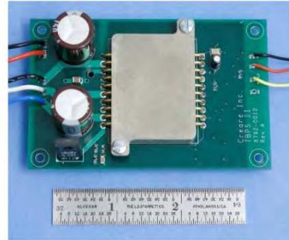
Microelectronic Compressor Motor Drive Electronics
