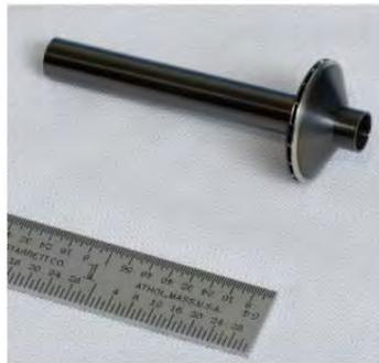
400 W Compressor Rotor with Hard Wear-Resistant Coating
