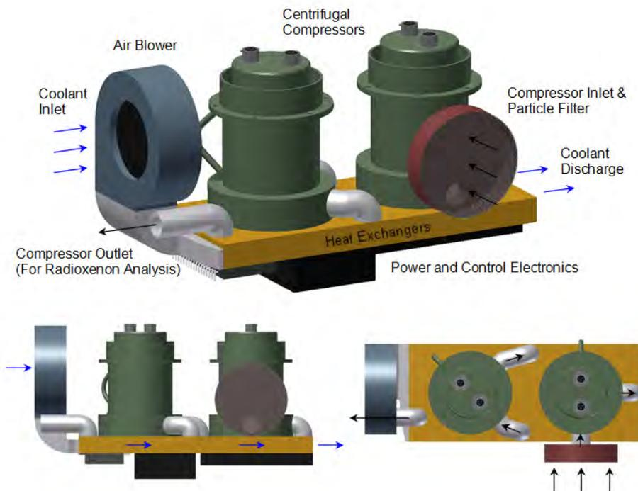
**Figure 1. Compressor system conceptual design.**
