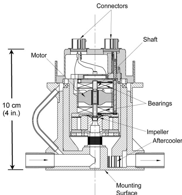
**Figure 4. Existing design for 160 W centrifugal compressor.**
