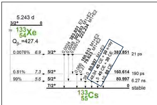
**Figure 1. The  $\gamma$ -ray level scheme for  $^{133}\text{Xe}$  with three additional decay paths included boxed in blue. The first number in the diagonal labels is the branching ratio, which is the probability of that particular decay occurring. The second number is the energy or approximate energy of the particular decay. For the three boxed decays the additional information gives secondary radiation signatures that are in coincidence with the decay.**
