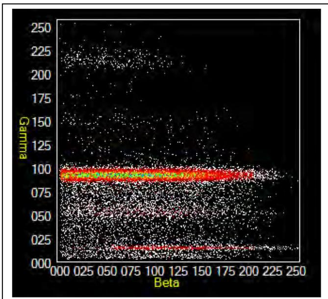
Figure 2. A  $\beta$ - $\gamma$  coincidence plot of the  $^{135}\text{Xe}$  calibration sample data.
