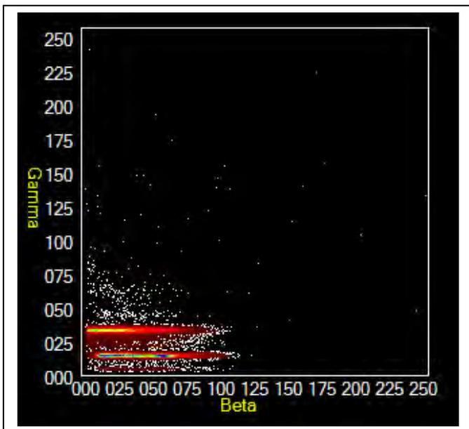
Figure 3. A  $\beta$ - $\gamma$  coincidence plot of the  $^{133\text{m}}\text{Xe}$  calibration sample data. The region circled in blue is the  $^{133\text{m}}\text{Xe}$  peak, with the other horizontal peaks being  $^{133}\text{Xe}$ .
