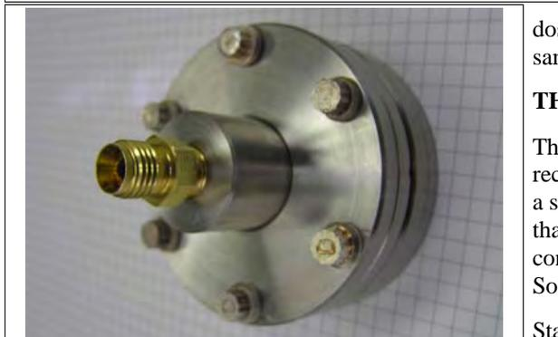
Figure 6: Chamber for dosing BC-404 with Rn.
