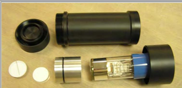
Figure 9: Memory effect test jig parts, disassembled.
