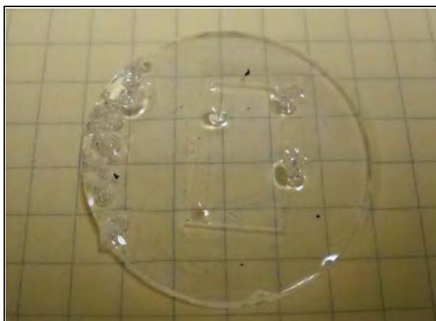
Figure 2: Bubbled 125 °C BC-404 sample.
