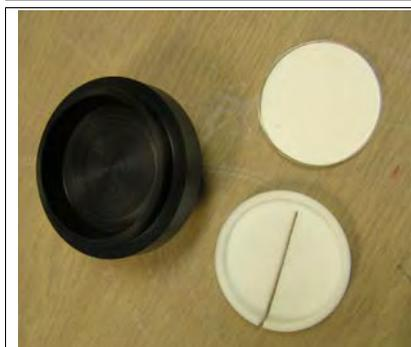
Figure 10: Sample mounting parts.
