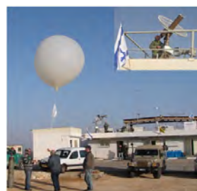
Figure 10. Launching the radiosonde and tracing by a radio-theodolite.
