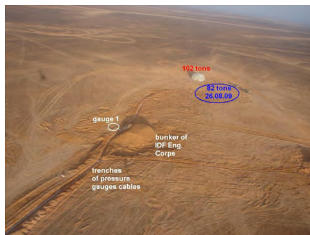
Figure 2. View of the main 102 ton charge assembled of four layers of big bags, with measured dimensions: base 8 × 8 m, height 4 m (a), and the small charge 10 tons, remote by distance 655 m (b).
