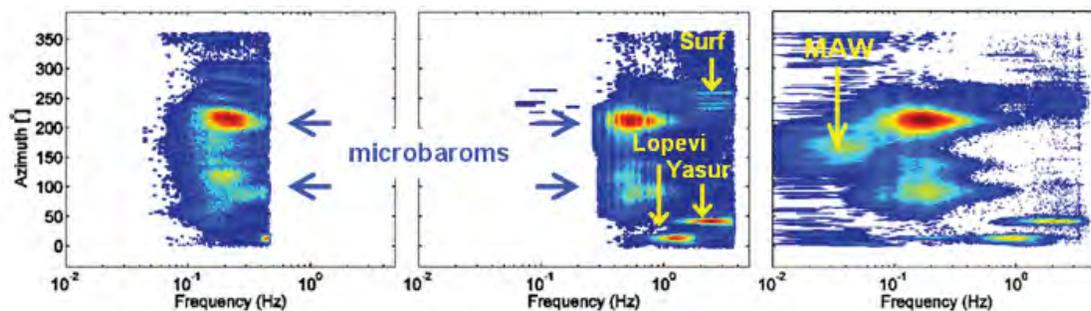
**Figure 3. Comparison between processing results using two 10-band low- (0.02-0.5 Hz) and high-frequency (0.1-4 Hz) configurations (left and middle, respectively) and a 15-band log-spaced configuration (0.01-5 Hz, right). Warm colors correspond to increasing number of detections in frequency-azimuth space.**
