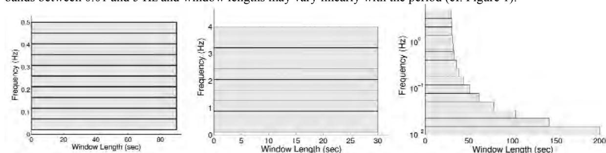
**Figure 1. Examples of two 10-band standard configurations for low- and high-frequency processing (0.02-0.5 Hz and 0.1-4 Hz, left and middle respectively), replaced by a single configuration consisting of 15 bands with log-spaced filter parameters (0.01-5 Hz) and a variable window length.**
