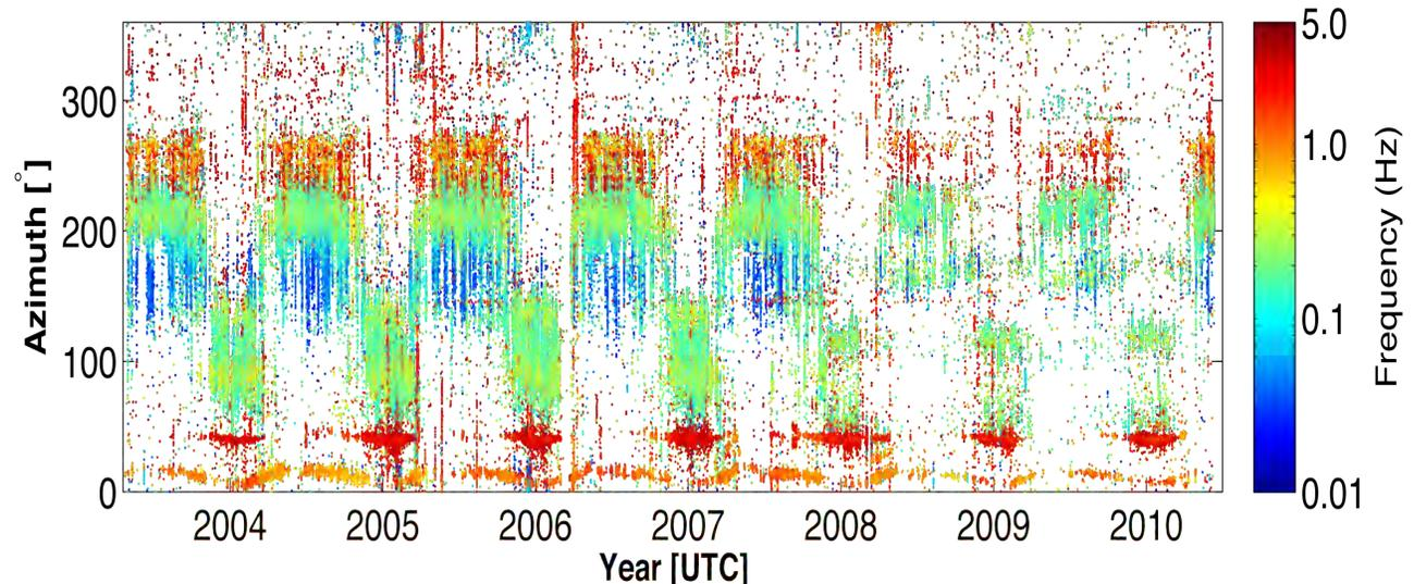
**Figure 4. PMCC detections at IS22 from 2003 to 2010 using the 15-band log-scaled filter parameters (0.01-5 Hz) and variable window length illustrated in Figure 1. From 2008 to 2011, the reduced detection capability is explained by a missing central array element.**
