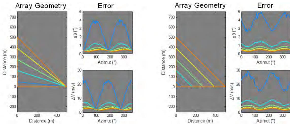
**Figure 2. Errors related to the geometry (flatness on the left, aperture on the right) of an array composed of 3 sensors with a sampling rate of 20 Hz.**
