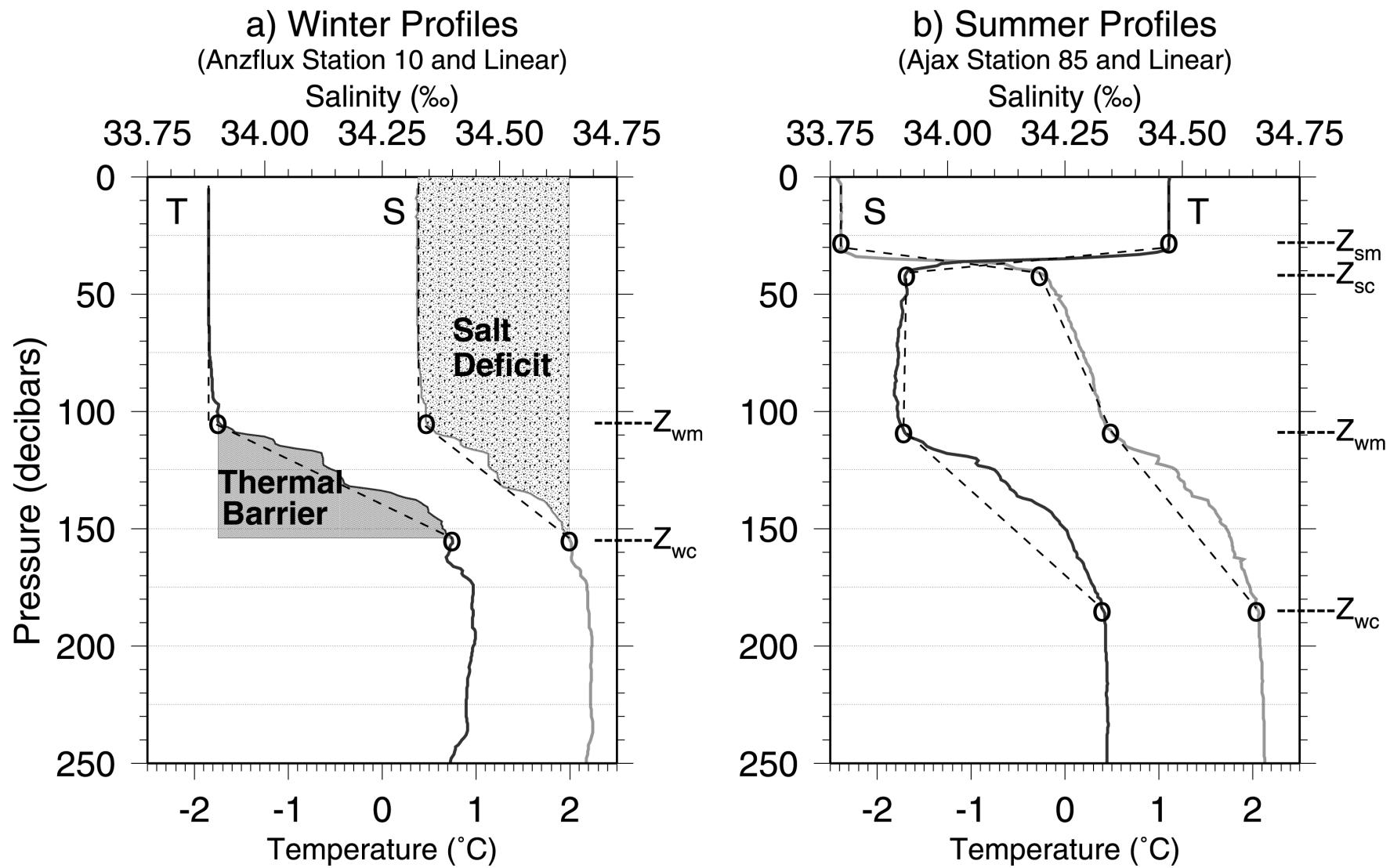
**Figure 1:** Ideal summer and winter profiles of T and S. Dashed line shows ideal profile shapes; shading indicates the area integrated to produce the Thermal Barrier and Salt Deficit for winter profiles. Key integration depths referred to in the text are also indicated.
