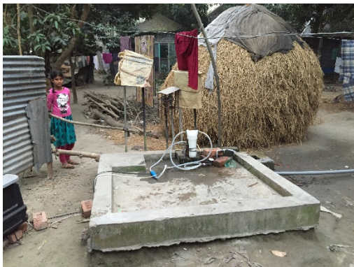
Figure 1. Field Site in Bangladesh. This is an 800 foot deep well that is low in arsenic. However the radiocarbon dates of the dissolved organic carbon are significantly younger than the dissolved inorganic carbon indicating intrusion of young, reactive groundwater. .
