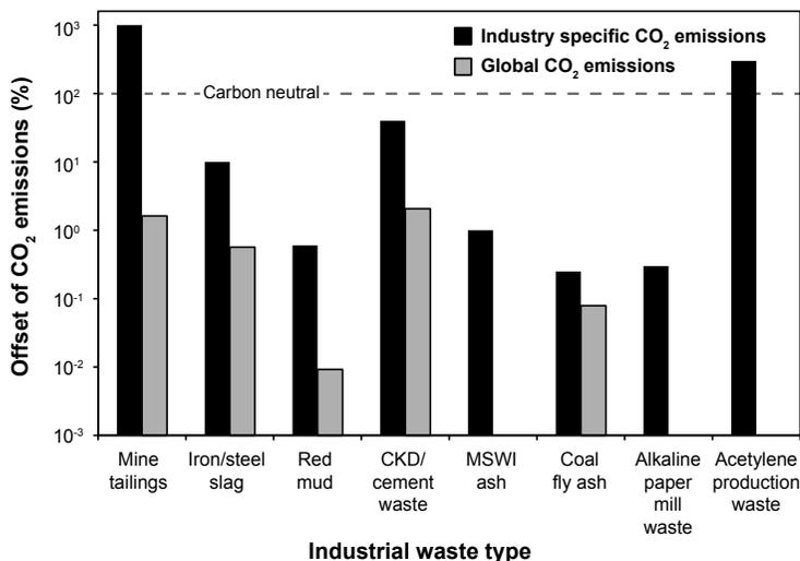
**Figure 10.** Percent offset of CO<sub>2</sub> emissions for specific industries and global annual emissions provided via carbonation of various industrial waste materials. CKD = cement kiln dust; MSWI = municipal solid waste incinerator. The data were insufficient to calculate the offset of total annual global CO<sub>2</sub> emissions provided via carbonation of MSWI ash, acetylene production, and alkaline paper mill waste.
