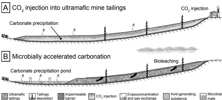
**Figure 7.** A schematic of two mine tailings facilities depicting (A) an abiotic strategy employing  $\text{CO}_2$  injection, and (B) use of bioreaching and microbial carbonate precipitation as strategies for carbon mineralization (modified after Power et al. 2013b).
