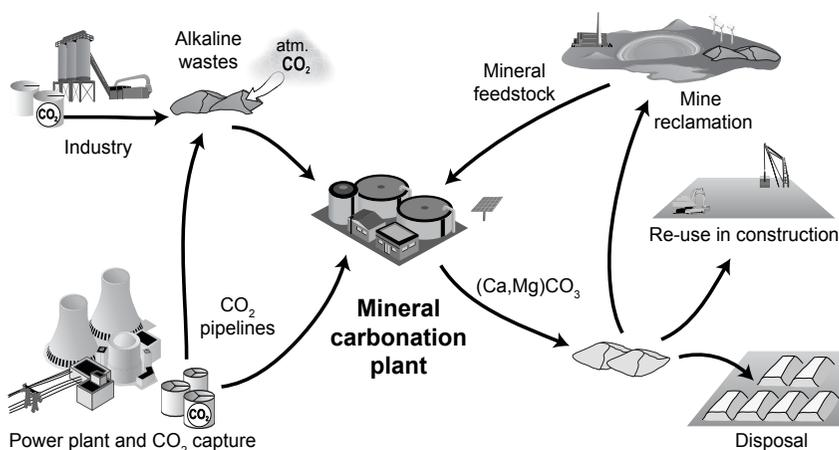
**Figure 9.** Material fluxes and processes associated with industrial carbonation of mineral feedstock and industrial alkaline wastes (modified after IPCC 2005). Graphical elements are courtesy of the Integration and Application Network, University of Maryland Center for Environmental Sciences ([ian.umces.edu/symbols](http://ian.umces.edu/symbols)).
