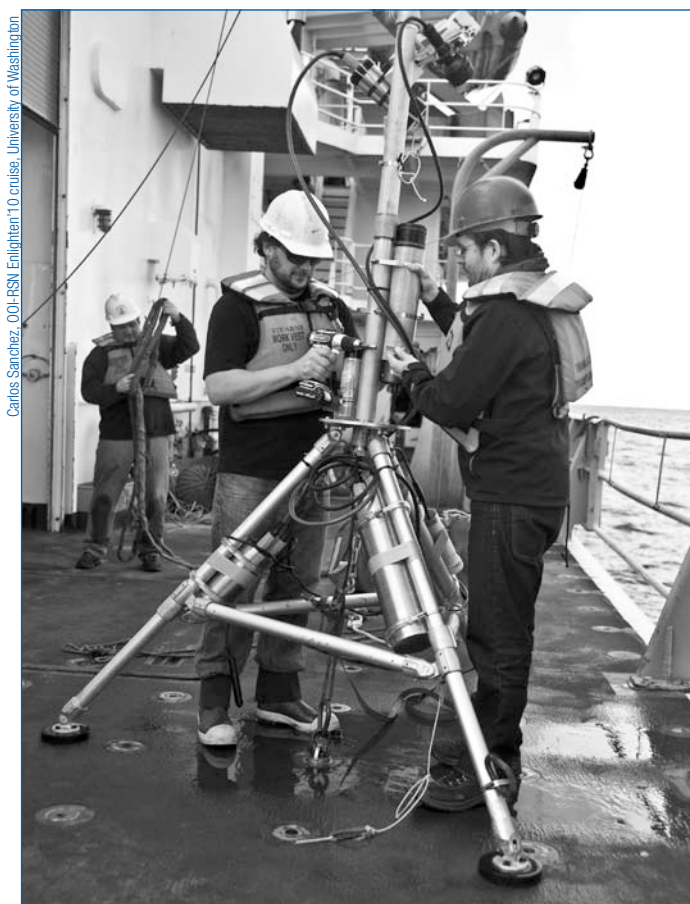
Crone and University of Washington graduate student Hugo Solis prepare the VentCam tripod for deployment at Axial Seamount on the Juan de Fuca Ridge.
