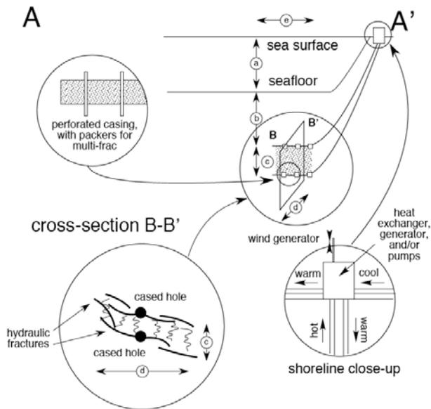
**Figure A3-1:** Notional design of shoreline installation for capture and storage of CO<sub>2</sub> from thermal convection of seawater through sub-seafloor peridotite via thermal convection, with low-grade geothermal power as a by-product.
