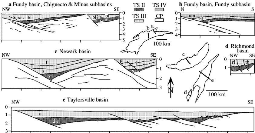
Figure 7 Representative cross sections of basins based on industry seismic profiles. Profile lines *a* (Fundy basin and Chignecto and Minas subbasins) and *b* (Fundy basin and subbasin) are adapted from Withjack et al (1995); *c* (Newark basin), revised interpretation based on Costain & Coruh (1989); *d* (Richmond basin), adapted from Cornet & Olsen (1990); and *e* (Taylorsville basin), based on a variety of unpublished seismic profiles and Milici et al (1991).
