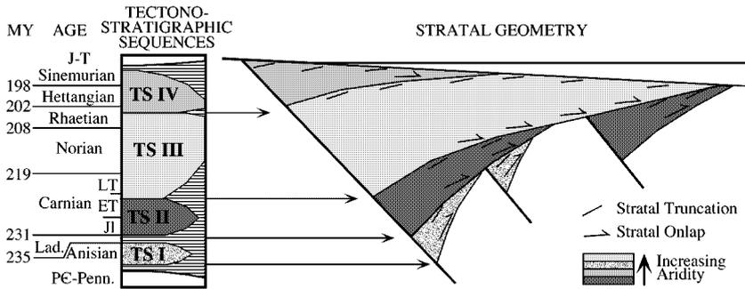
Figure 9 Basic tectonostratigraphic sequences of CAM basins based largely on seismic profiles and coring.
