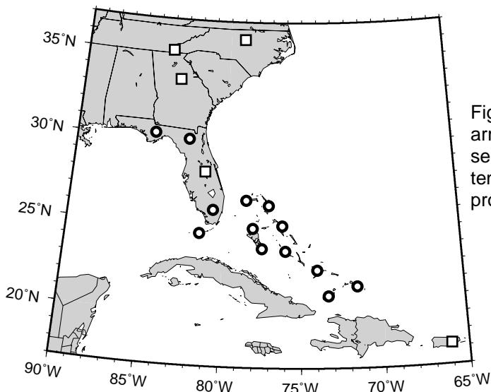
Figure 4. Schematic map of the proposed array. Squares show permanent broad-band seismic observatories, circles indicate tentative locations for the nodes of the proposed temporary array.
