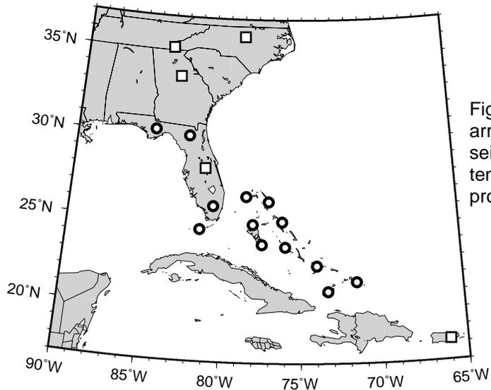
Figure 4. Schematic map of the proposed array. Squares show permanent broad-band seismic observatories, circles indicate tentative locations for the nodes of the proposed temporary array.
