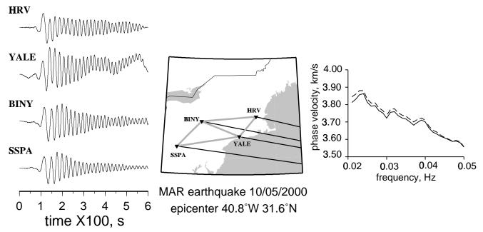
Figure 5. (left) Well-dispersed Raleigh wave from a Mid-Atlantic Ridge earthquake observed on four vertical-component broadband stations in Northeastern US. (middle) Map showing four stations (HRV, YALE, BING, SSPA), which define southern and northern trianges. (right) Local estimate if phase velocity for each triangle, computed with the differential phase method. Note that the northern triangle (solid curve) has systematically lower velocities.
