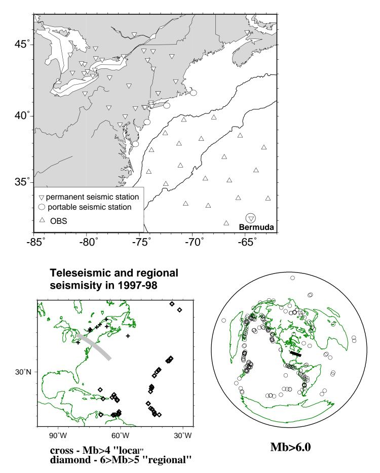
Figure 3. (TOP) A map of existing permanent seismic observatories in northeastern North America and on Bermuda (inverted triangles), and a tentative scematic of the proposed deployment (circles and triangles). (BOTTOM) Seismic activity in a 2-year period (1997-98) illustrates the likely distribution of sources the proposed array will observe.
