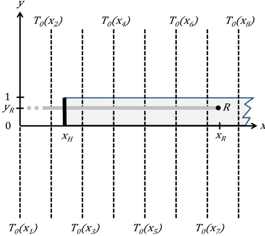
Fig.1. Surfaces of equal travel time (dotted vertical lines); heterogeneity (bold vertical bar at  $x_H$ ). Region of constant travel time perturbation (grey rectangle); receiver (circle  $R$  at  $x_R$ ); line segment along which the adjoint field  $\lambda$  is non-zero
