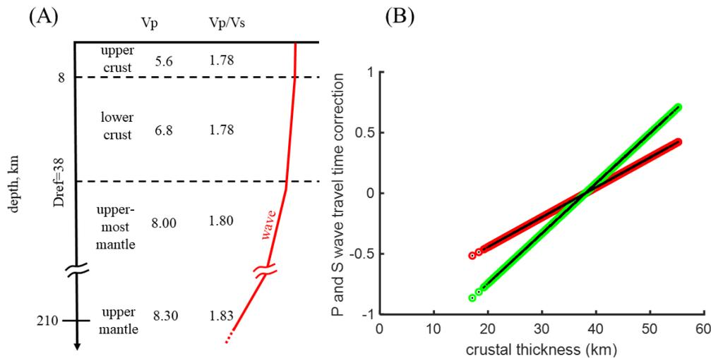
Fig. 1. (A) Earth model. (B) Calculated travel time corrections  $\Delta T_P$  (red) and  $\Delta T_S$  (green) and best-fit straight lines.
