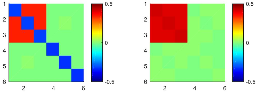
Figure 2. The two unresolved linear combinations of elastic parameters for a “both  $X$  and  $V$ ” inversion, here shown as  $6 \times 6$  Voigt matrices  $C_{ij}$ . They correspond to two different linear combinations of the Lamé parameters  $\lambda$  and  $\mu$ . Only the elements  $C_{14}$ ,  $C_{15}$ ,  $C_{16}$ ,  $C_{24}$ ,  $C_{25}$ ,  $C_{26}$ ,  $C_{34}$ ,  $C_{35}$ ,  $C_{36}$ ,  $C_{45}$ ,  $C_{46}$  and  $C_{56}$  are fully-resolved.
