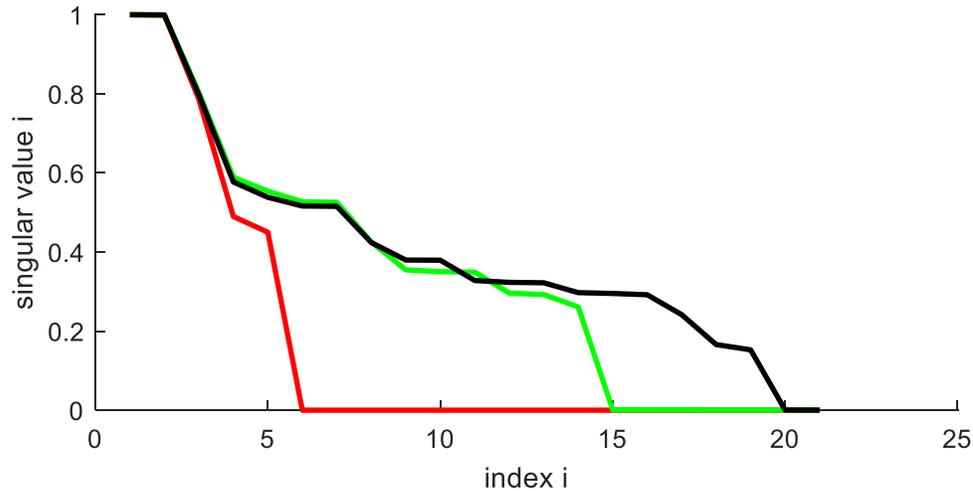
Figure 1. Singular values, normalized and sorted by size. (Red)  $X$  only, (green)  $V$  only, (black) both  $X$  and  $V$ . Two choices of isotropic medium, with Lamé coefficients  $(\lambda, \mu)$  of (1.1,1) and (2.1,1), respectively, gave this same result.
