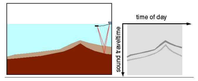
After several hours, a complete image, or **seismic profile** of the seafloor is made. Note that this image differs from a true geological cross-section in several ways:
