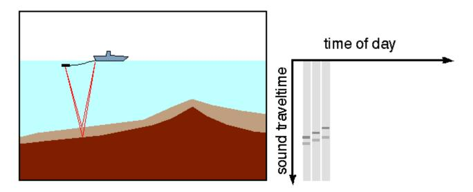
After 30-60 seconds, the air gun is detonated again, and the measurement and plotting process is repeated, with each stripe being drawn slighly to the right of previous stripes. Note that the time of the reflections is different, since the depth to the rock layers change as the ship moves.
