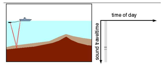
A sound wave (red line) is created by an "air gun" on the ship. The sound travels down through the water (blue), and penetrates into the layers of sediments (light brown) and rocks (dark brown) of the ocean floor. Some of this sound reflects (echos) off the layers, and travels back up to the surface of the ocean, where it is recorded by a hydrophone (black bar) trailed behind the ship.
