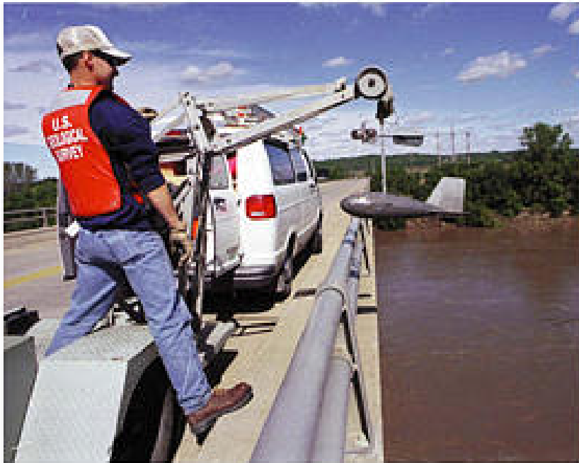
Discharge measurements made during floods are used to develop stage-discharge relations at each gaging station. (Photograph, Lawrence Journal World, Lawrence, Kans.)
