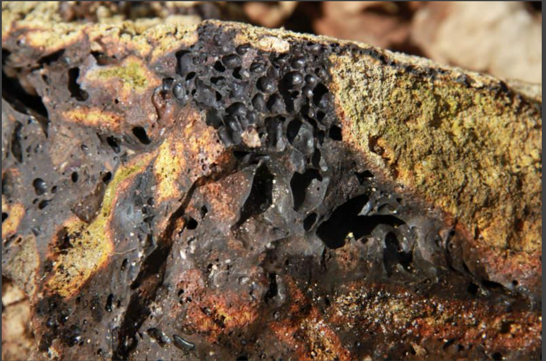
Slag (waste product of refining process)
