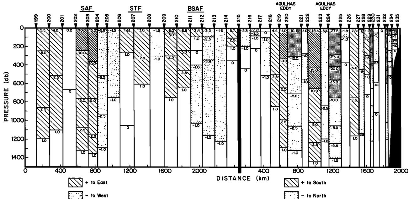
Fig. 3. Geostrophic speeds crossing the SAVE 4 section relative to a 1500-dbar zero reference level. For the continental margin stations where the seafloor is shallower than 1500 dbar, the flow at the seafloor is taken as zero. The Benguela-South Atlantic front (BSAF); subtropical front (STF), and subantarctic front (SAF) are labeled.
