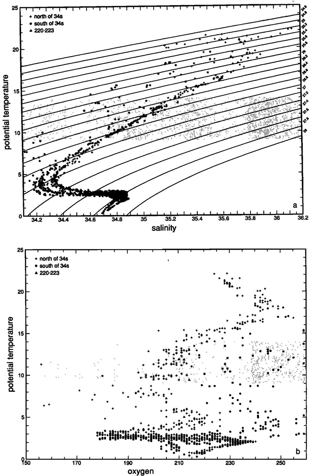
Fig. 5. Potential temperature versus (a) salinity in parts per thousand, (b) oxygen in micromoles per kilogram, and (c) chlorofluoromethane 11 and (d) chlorofluoromethane 12 in picomoles per kilogram for the SAVE stations shown in Figure 1. The 9°–14°C thermocline stratum is stippled.
