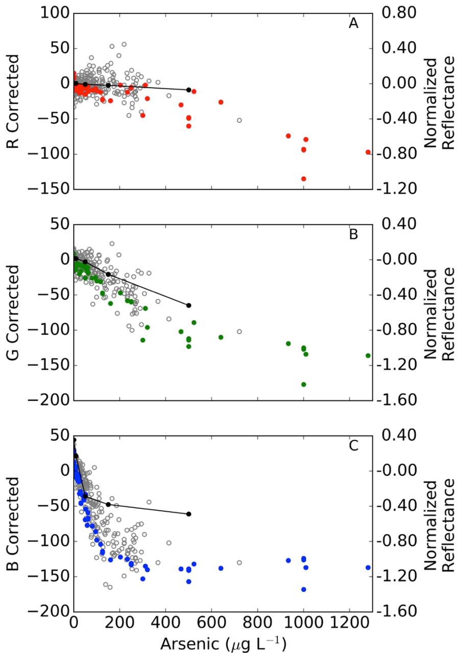
Figure 2: Cross validation plot of photo-predicted As concentration compared with lab-measured As concentrations in laboratory samples (red) and field samples (blue) using a single, combined multiple regression model of Photoshop-extracted RGB color data.
