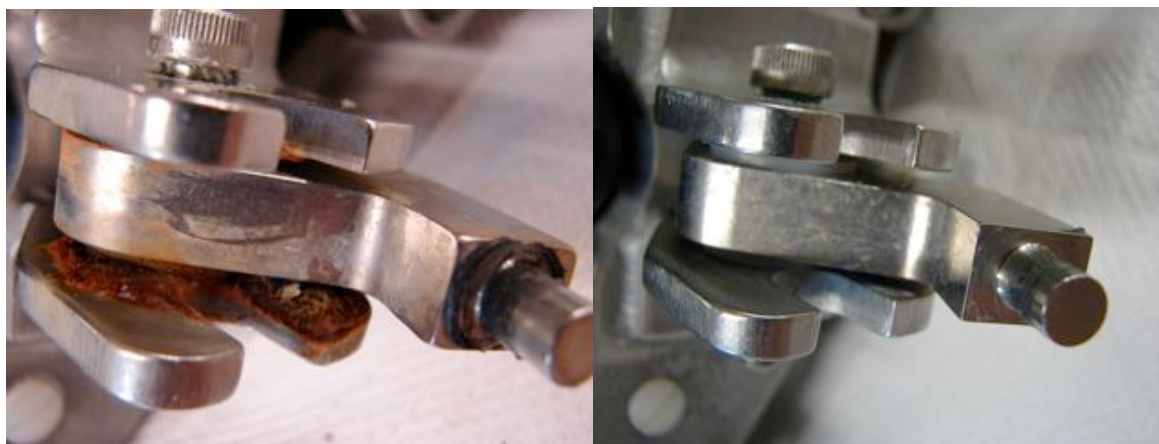
Figure 24 Corrosion on release lever and clevis of sn 31097 (left). An uncorroded release sn 31117 (right) shown for comparison.
