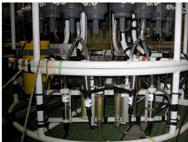
Figure 4 . Left: CTD primary and secondary sensor arrays and Y-tube water pump system. Right: sampling for oxygen content.
