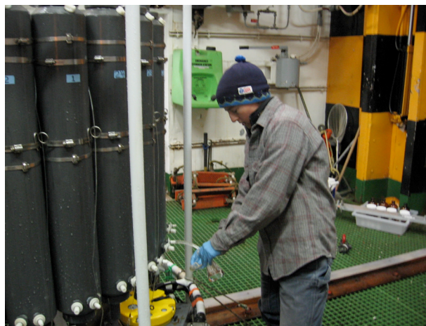
Figure 4 . Left: CTD primary and secondary sensor arrays and Y-tube water pump system. Right: sampling for oxygen content.
