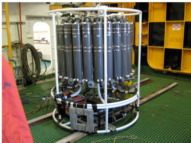
Figure 3 The CTD and niskin rosette fish. Left: on deck in Baltic Room. Right: during deployment.
