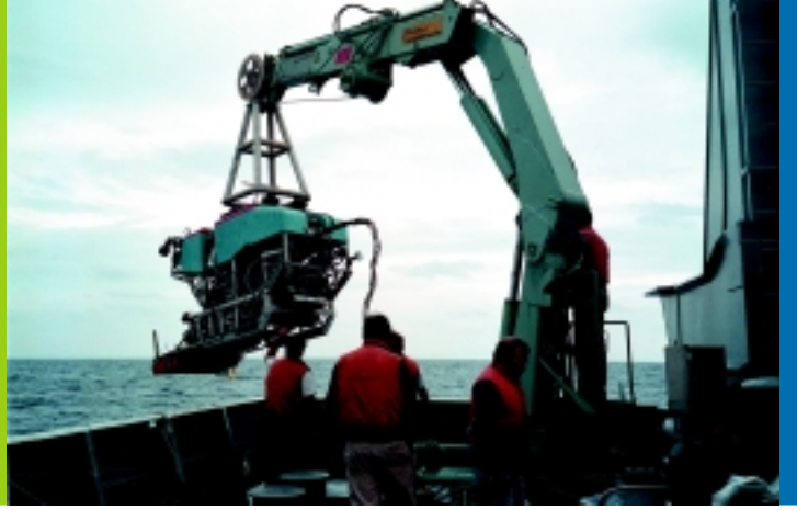
Figure 16. The remotely operated vehicle, Jason , is being deployed. The fiber-optic cable permits the shipboard pilot to navigate Jason , and also to transmit data back from the seafloor in real time for analysis. Photo courtesy of Woods Hole Oceanographic Institution.
