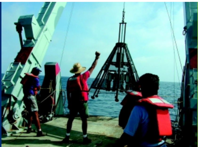
Figure 25. Here, Oregon State University's multicore system, deployed from the R/V Melville , is recovered full of mud. This device lands gently on the seafloor, then penetrates about 50 cm before closing trap doors to safely recover multiple pristine samples of the sediment-water interface. Recovery often reveals living tube worms or shrimp—somewhat startled but essentially undisturbed. Such sampling devices offer an unique glimpse of life at the seafloor and the chemical transformations that occur as newly fallen biogenic debris is converted into the sedimentary record. Photo courtesy of A. Mix, Oregon State University and M. Lyle, Boise State University.
