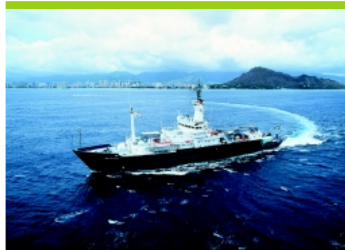
Figure 3. The Global Class R/V Melville , built in the 1969 and re-engined, stretched, and upgraded in 1991, will be retired in 2014.
