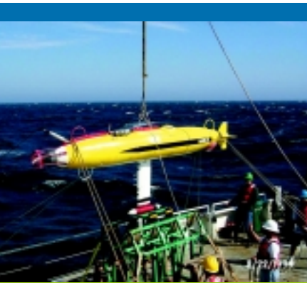
Figure 10. MARLIN, the research instrument deployed here from the R/V Wecoma off the coast of Oregon, is a sophisticated towed body capable of making measurements of velocity shear, turbulence, and fine structure to depths of 3400 m. The purpose of the instrument is to investigate physical processes that lead to mixing of the deep ocean near topography such as seamounts, submarine canyons, escarpments, and mid-ocean ridges. Photo from http://mixing.oce.orst.edu/Photogallery/Marlin/start.htm .
