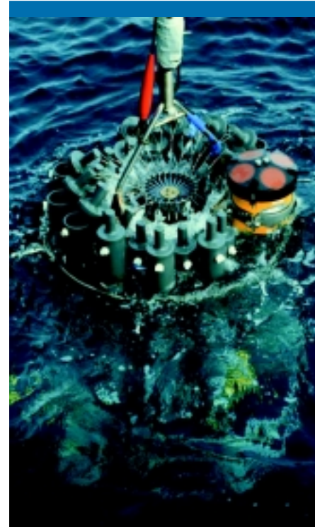
Figure 19. A CTD (Conductivity, Temperature, Depth) instrument being deployed from the R/V Oceanus in the Irminger Sea (east of Greenland) to study the circulation and convection there. During the cruise, scientists did a basin-wide CTD survey of the sea, and deployed two “profiling CTD moorings.” Photo by C. A. Linder, Woods Hole Oceanographic Institution.
