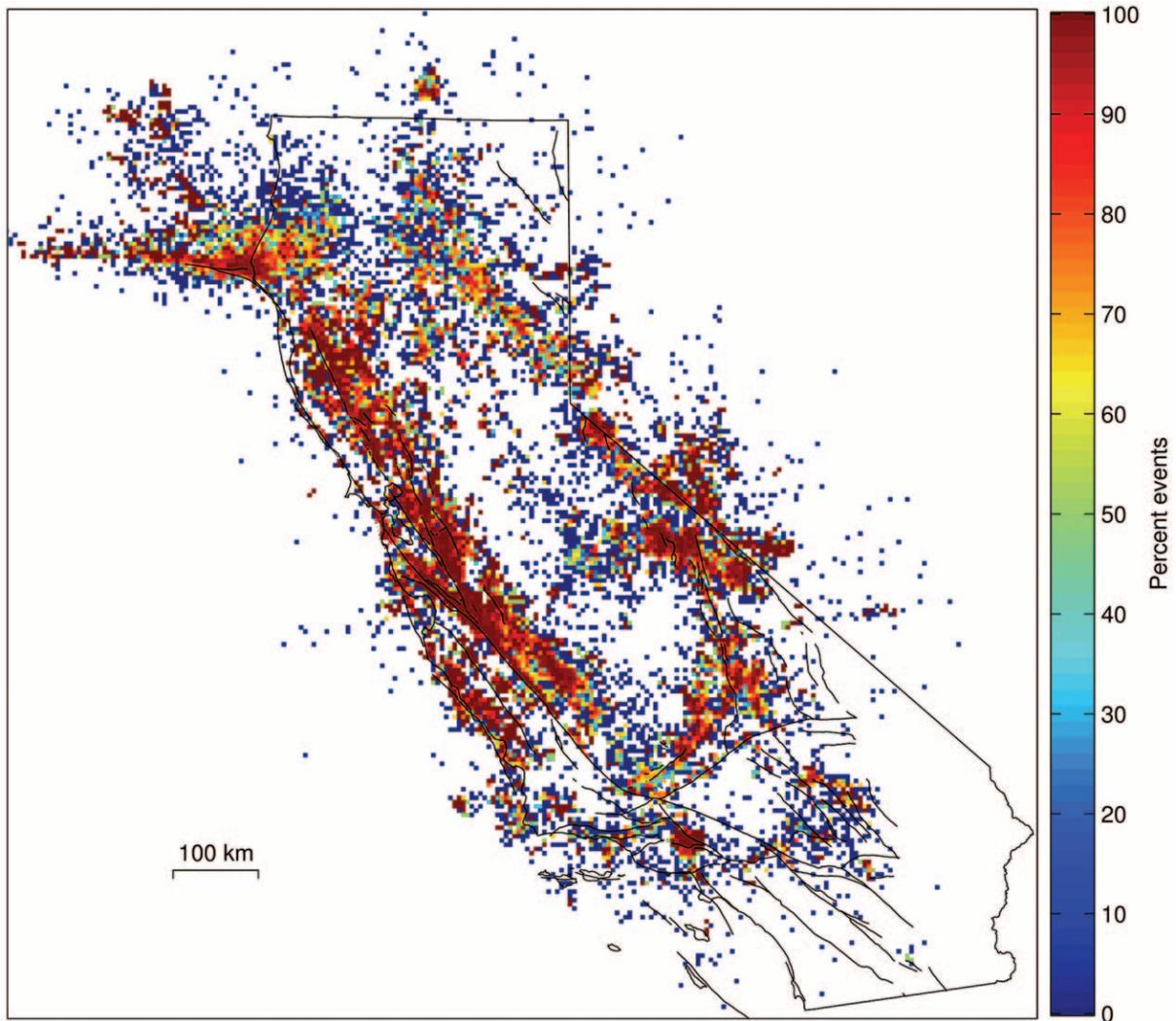
Figure 5. Percentage of correlated events that have cross-correlation coefficients of  $CC \geq 0.7$  with at least one other event recorded at four or more stations. Percentages are computed from the total number of events within bins of  $5 \times 5$  km.
