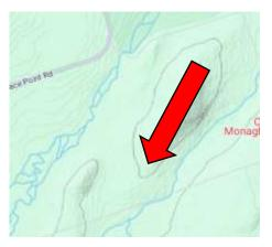
Step 4. Read the rectangle's rotation angle (in the 0-360 range) from the Formal Shape menu. You need to be careful that you're not 180 degrees off with the angle. In this example, the downslope direction is N208E
