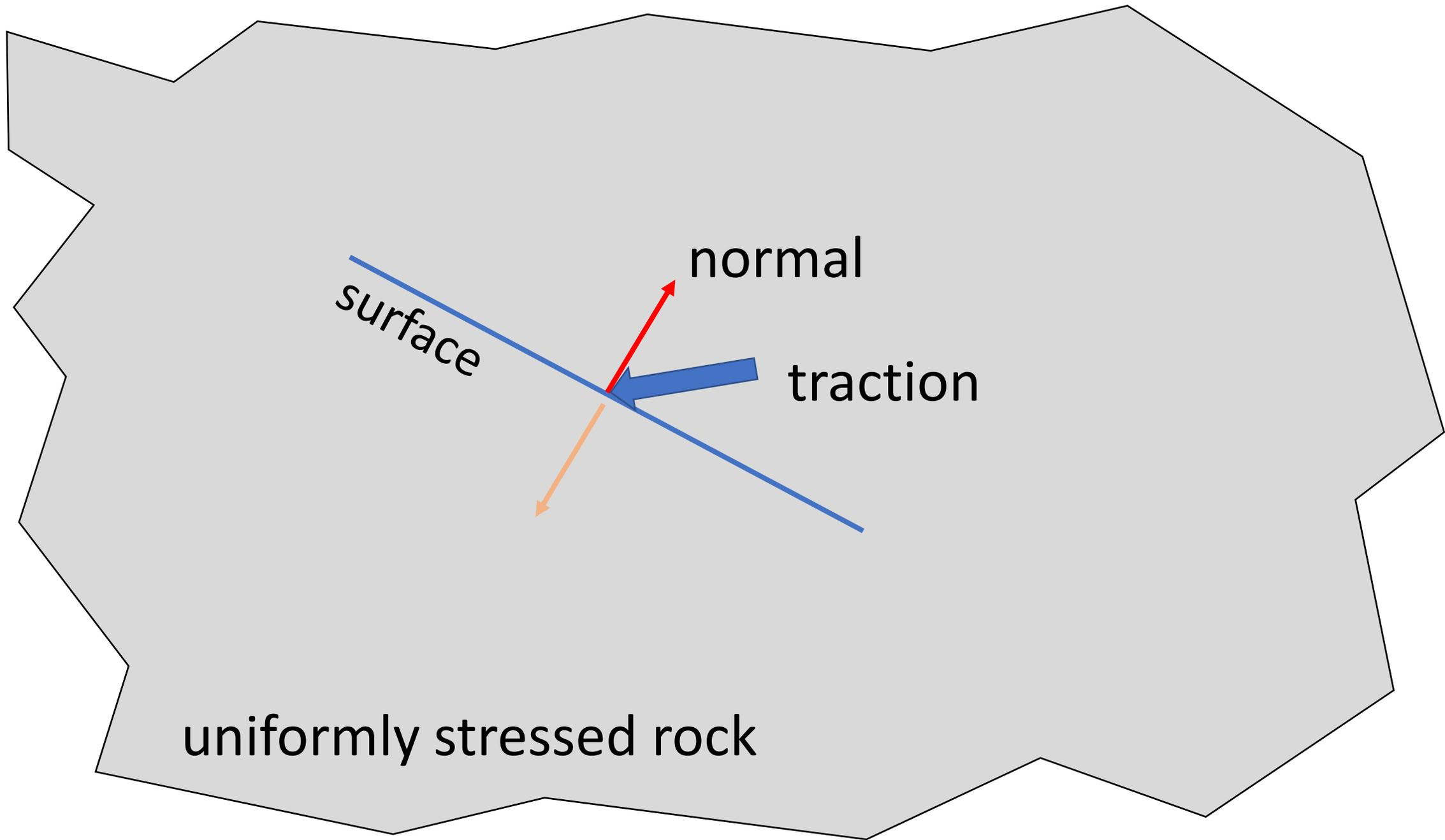
Tractions on two sides of a surface
