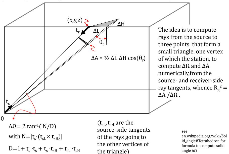
The amplitude of a body wave is proportional to 1/Rg
